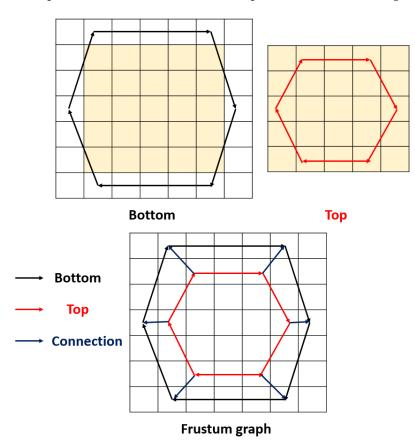
Figure 2. The bottom, top, and frustum graphs used to create the frustum pattern.
