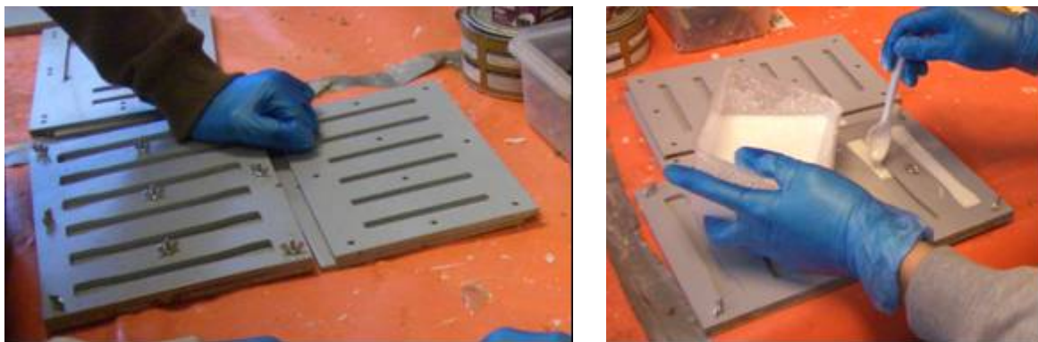
Figure 3.4 : Composite mixture poured into the moulds
