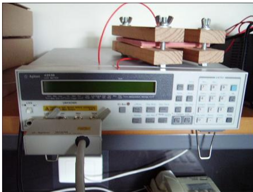
Figure 3.8: Parallel plated method set up
