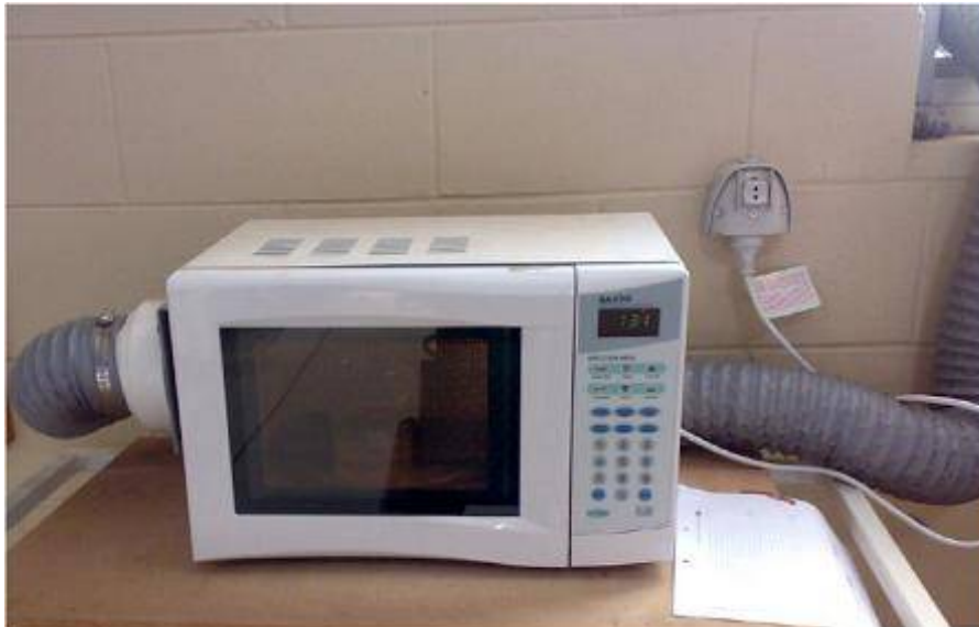
Figure 3.5 : SANYO 800 W microwave with attached air duct
