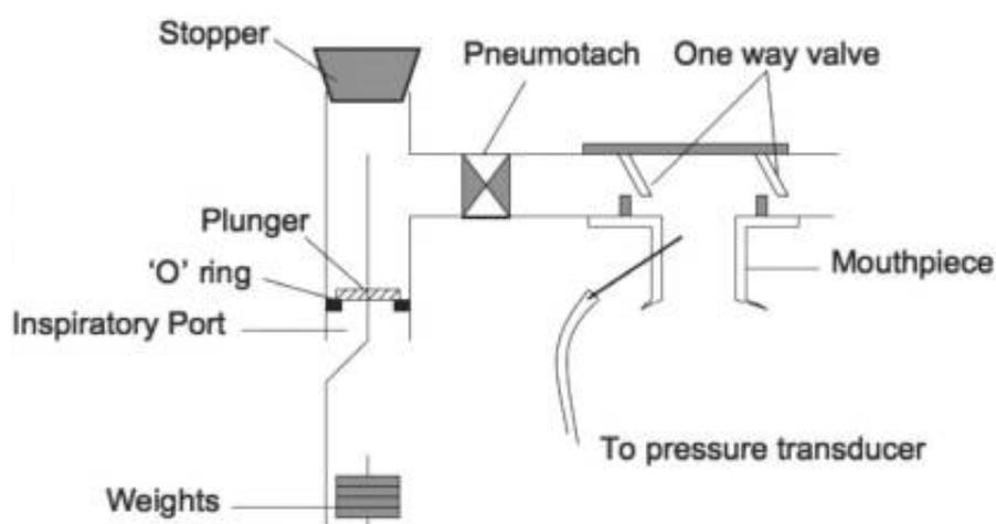
**Figure 2.10** Schematic of inspiratory pressure threshold loading device [130].
