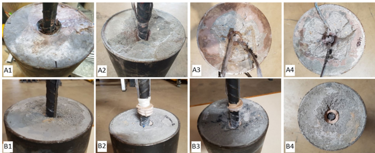
Fig. 16 Cone-shape damage at the loading end of the specimens with different embedment lengths
