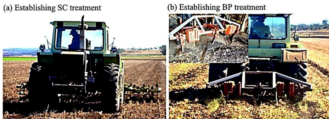
Figure 5.2: Establishment of two renovation treatments for 2010 wheat crop after 2009 soybean harvest at site A1, Marinya farm, Cambooya, Australia
