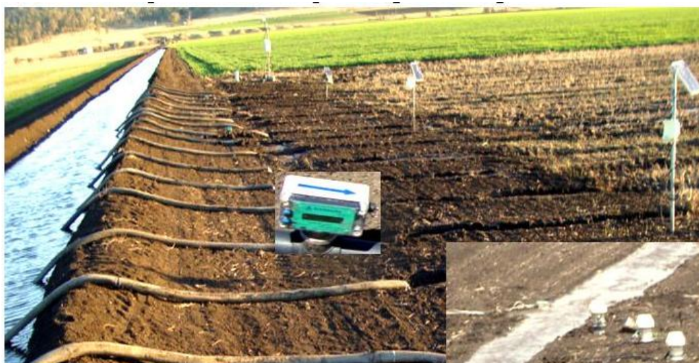
Figure 5.4: Overbank systems and IRRIMATE™ meters for measuring inflow rate. Insert shows water advance sensors and soil moisture sensors layout during irrigation. Photo taken during 2010 wheat season at site A1, Cambooya, Australia
