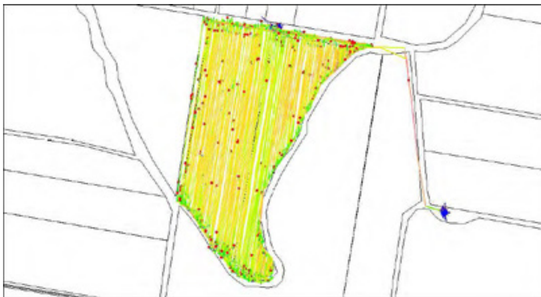
Figure 2.10 GPS harvester tracks in a harvested field, coloured by speed (Beattie and Crossley 2006)
