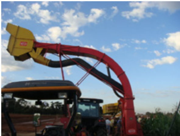
Figure 4.4 Attachments are available for choppers and forage harvesters to remove a proportion of the leaf and lighter material.
