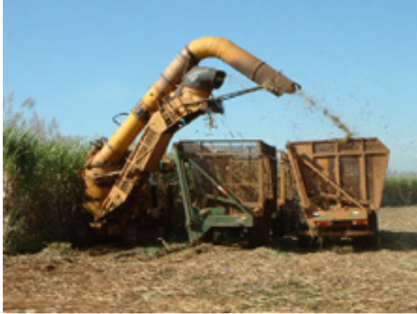
Figure 4.3 System in Brazil for separating trash on the harvester and transporting it separately to the mill.
