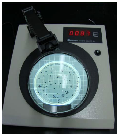
Figure 3-2 SUNTEX colony counter
