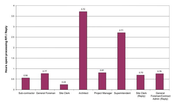
Figure 8: Estimated mean cycle times for processing RFIs and site instructions (EDMT)
