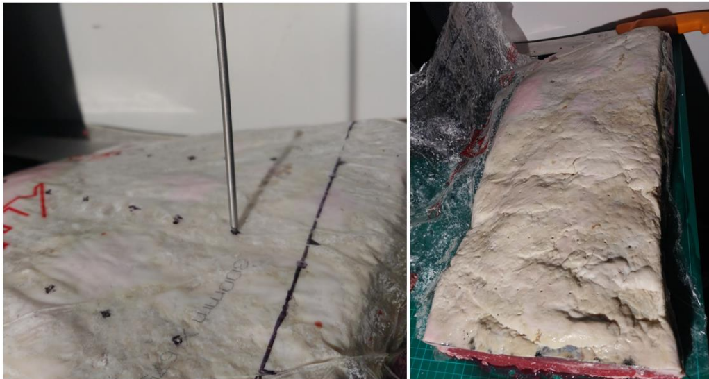
Figure 5-12: Marking nodes through plastic wrapping using a stainless-steel skewer.
