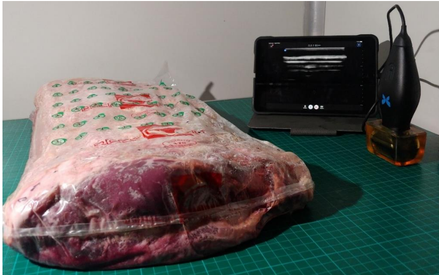
Figure 5-11: Experimental set-up for B-Mode ultrasound sensing experiment.
