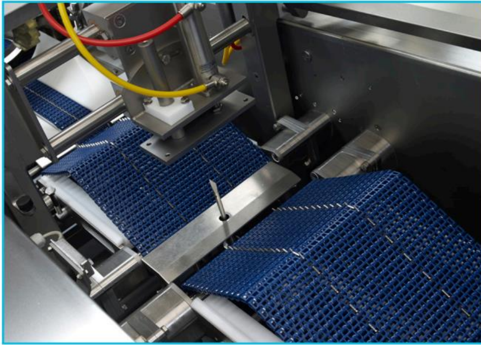
Figure 2-19: The optical probe (spike at centre of image) for acquiring fat depth of the pork primal for adjusting the trimming depth of Frontmatec's automatic loin trimmer. Source – (Frontmatic, 2020a)
