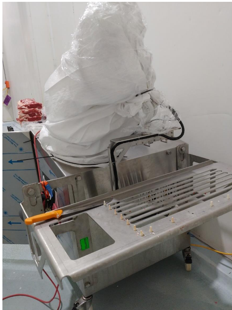
Figure 6-6: The experimental setup inside the collaborating processor's facility using a manipulator arm robot to position sensors at measurement nodes.
