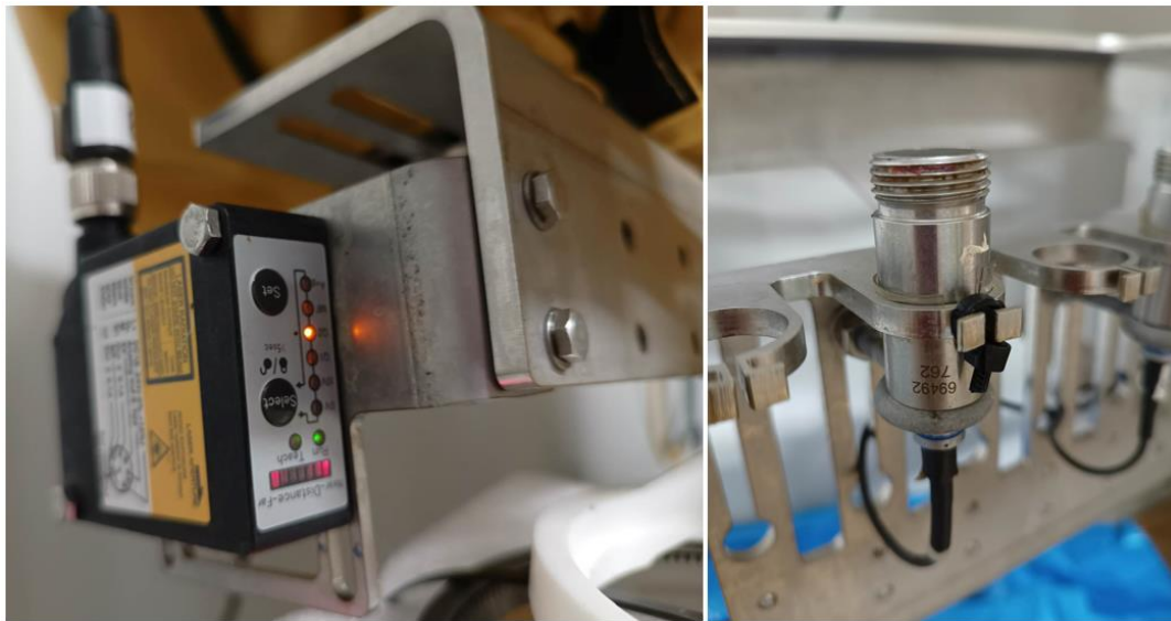
Figure 6-9: LiDAR and ultrasound sensors assembled onto the C-Arm bracket.
