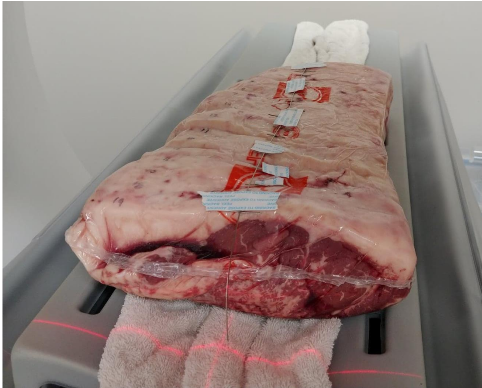
Figure 4-1: The laser lines of the CT imaging system were used to align to the front edge of the striploin (rump / cranial face) to align nodes to appear on similar cross-sectional images.
