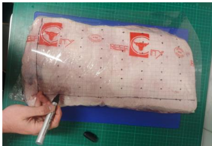
Figure 3-20: A clear, plastic grid was aligned with the origin and used to mark up the 25 mm X 50 mm spacings to create the node mesh on each striploin.
