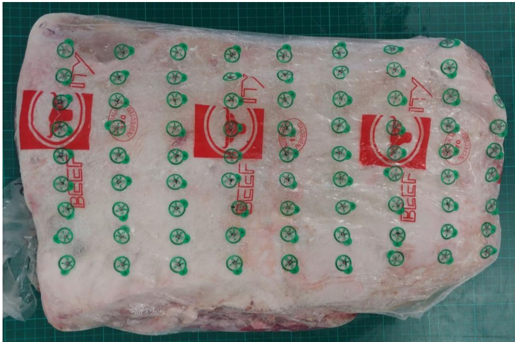
Figure 4-2: The adhesive CT markers were attached on the plastic at the locations of the prescribed measurement nodes.
