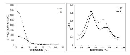
Figure 4. Thermal plots; (a) storage modulus vs temperature, and (b) Tan  $\delta$  vs temperature
