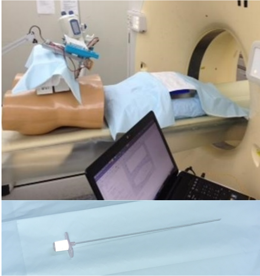
Figure 4.2: Top: System setup including infrared emitters, wii cameras fixed and a phantom with entry marks. Bottom: The biopsy needle with infrared reflective tape attached.
