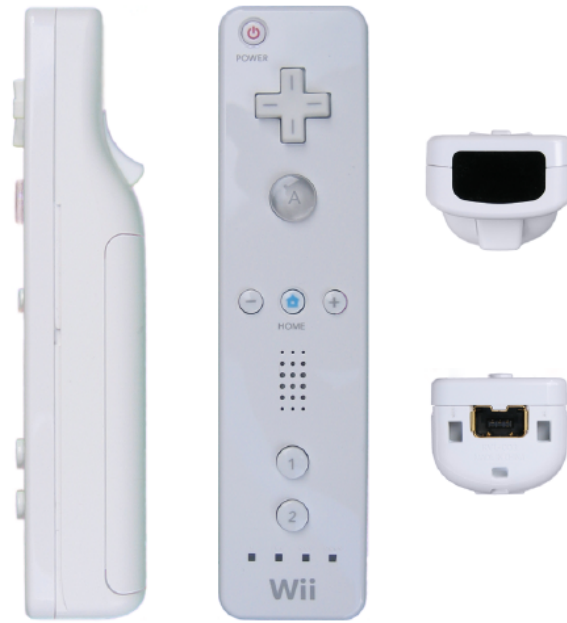
Figure 3.6: Nintendo Wii remote infrared camera used in this research (Lee 2008).
