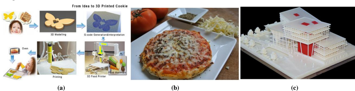
Figure 6: a) 3D food printing process of a customized cookie (Sun, et al., 2015), b) Printed Pizza by 3D Foodini printer (Keating, 2014) c) 3D printed building model (Meijs, 2013).
