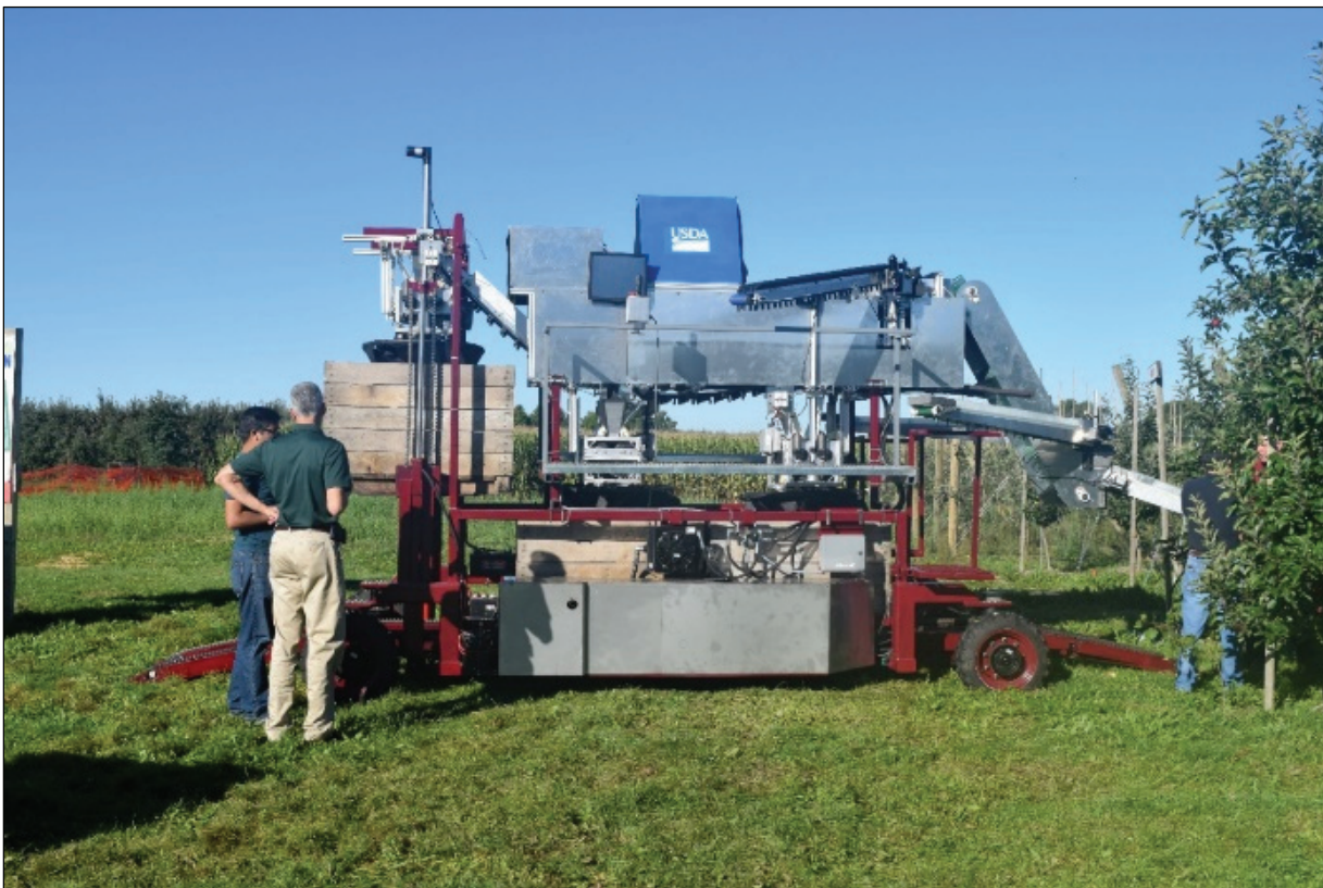
Figure 2. Apple harvest and in-field sorting machine prototype being tested in a commercial orchard in Michigan during the 2016 harvest season (Zhang et al., 2017c).
