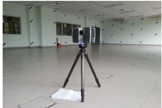
Figure 5. Experiment of scale effect in phase based scanner datum transformation
