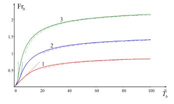
FIG. 4. The dependence of critical Froude number against the wave period  $\tilde{T}_b$ . Line  $1-\Omega=0$ , line  $2-\Omega=0.5$ , line  $3-\Omega=1$ . Dotted lines pertain to asymptotic dependences for small periods, whereas dashed lines pertain to asymptotic dependences for large periods.
