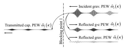
FIG. 6. Schematic illustration of one of the scenarios of blocking phenomenon for gravity-capillary waves. The incident wave gives rise to two reflected waves and one transmitted wave.
