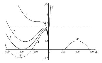
FIG. 5. Dimensionless frequency of upstream and downstream (line 0) propagating waves as a function of the dimensionless wavenumber as per Eq. (2) with  $\Omega = 0$  and  $S = 7.4 \times 10^{-6}$ . Lines 0 and 1 pertain to  $Fr = 5.67 \times 10^{-2}$ , line 2— $Fr = 7.0 \times 10^{-2}$ , line 3—Fr = Fr<sub>NEW</sub>  $\equiv \sqrt[4]{4S}$ , lines 4, 4', and 4" pertain to Fr = 7.75 × 10<sup>-2</sup>.
