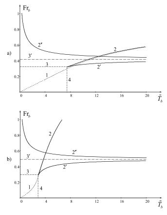
FIG. 8. The critical Froude number against the normalised wave period  $\tilde{T}_b$  for gravity-capillary surface waves with  $S = 7.4 \times 10^{-3}$ . Frame (a) pertains to  $\Omega = 0$ , and frame (b)—to  $\Omega = 1$ .
