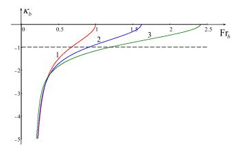
FIG. 3. The dependence of the blocking wavenumber  $\kappa_b$  against the critical Froude number  ${\rm Fr}_b$  at different vorticity parameters  $\Omega$ . Line  $1-\Omega=0$ , line  $2-\Omega=0.5$ , line  $3-\Omega=1$ .
