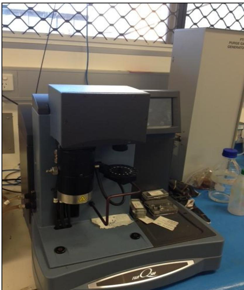
**Figure 3.5: TGA-Q500 Used for Thermal Property Analysis**
