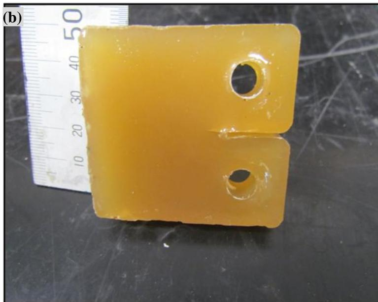
**Figure 3.14: (a) Tension Test and (b) Clevis Design Used for CT**
