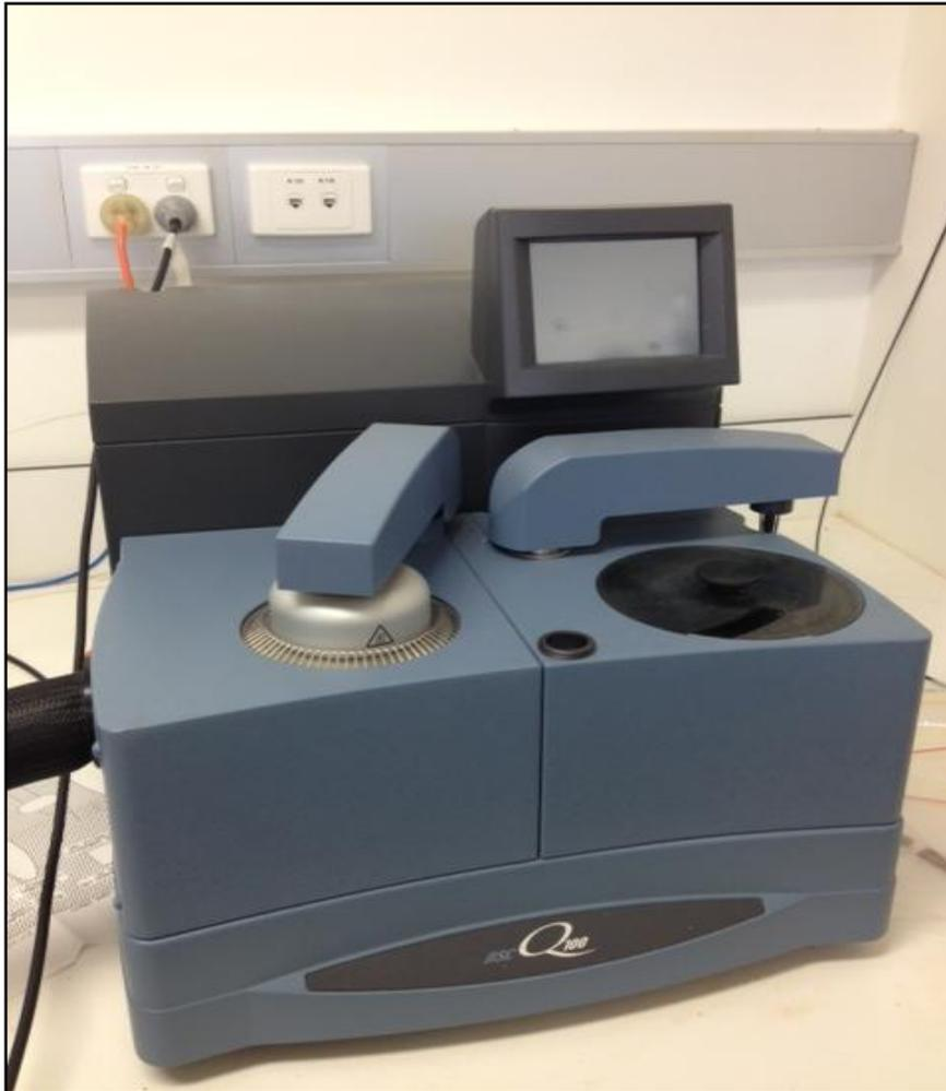
**Figure 3.6: Differential Scanning Calorimeter (DSC-Q200) Used in the Study**
