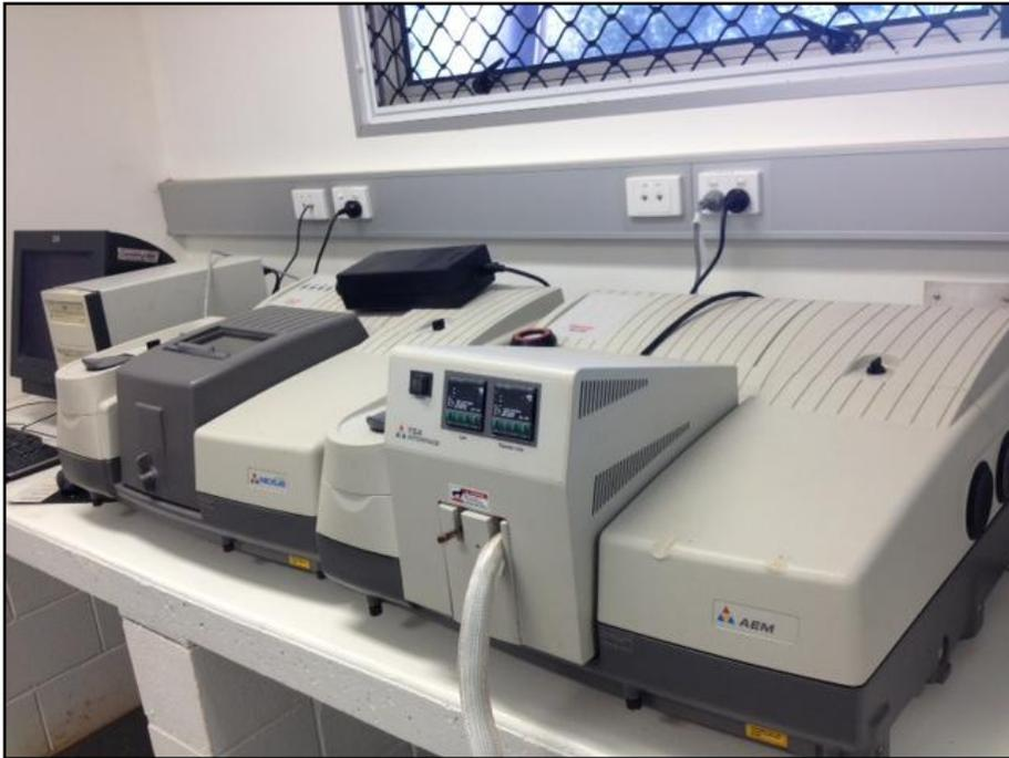
**Figure 3.4: FT-IR Spectrophotometer Used in the Study**
