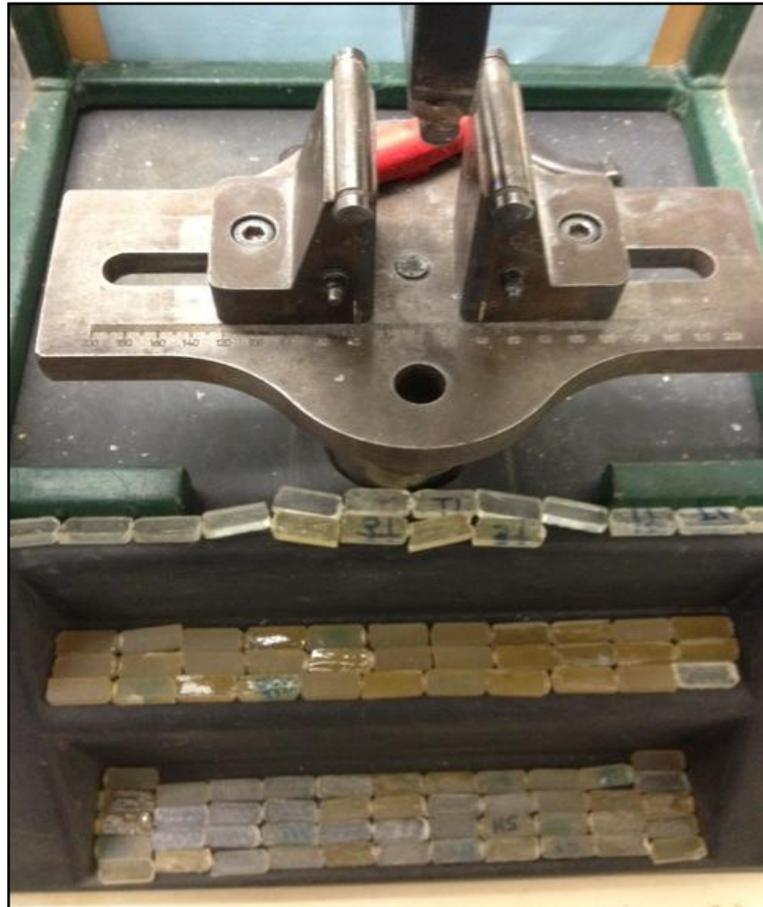
**Figure 3.9: Flexural Strength Testing Using MTS Universal Machine**
