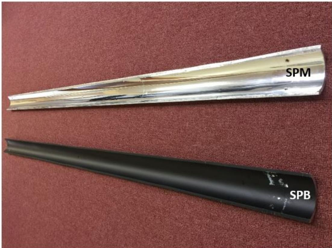
*Figure 3.13: Geometries of secondary parabola with mirror film (SPM) (upper) and secondary parabola painted black (SPB) (lower).*
