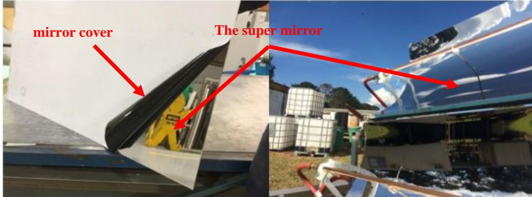
*Figure 3.2: Super mirror stainless steel grade 316 (left) and the installed mirrors of the solar heating system (right), consisting of two symmetrical parabola collectors.*
