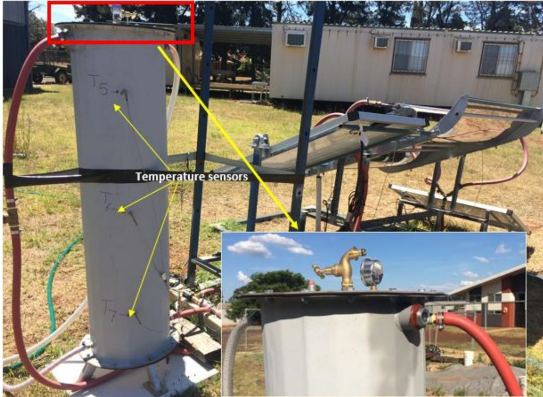
*Figure 3.20: Storage water tank before installing the thermal insulation, showing sites of water temperature sensors and zoomed on the tank cover showing the safety valve, pressure gauge, water tap and sight glass with hexagonal head.*
