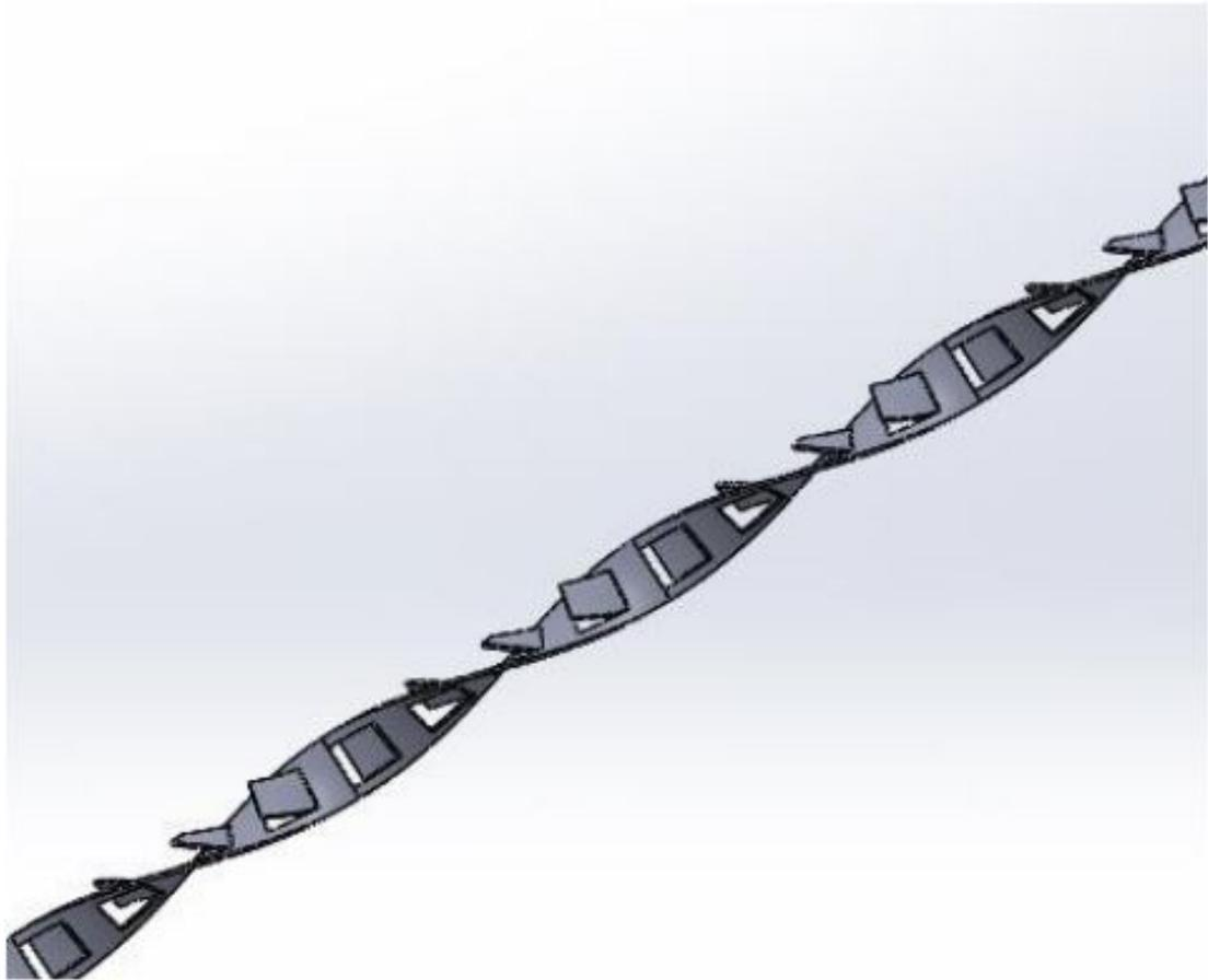
*Figure 2.43: Geometry of the Louvered twisted tape with perforations (Ghadirijafarbeigloo et al. 2014).*
