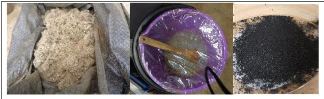
Figure 3.5: Materials (chopped CGW, gelatinised cassava starch, biochar)
