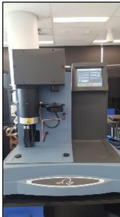
*Figure 4.2: Thermogravimetric Analyzer*
