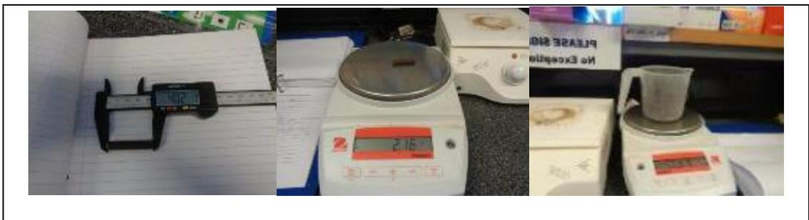
Figure 3.8: Instrumentation for measurement of the pellet size, weight and apparent density
