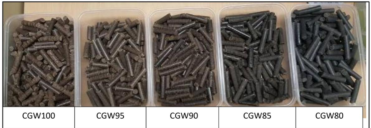
*Figure 3.7: CGW and CGW-biochar blended of pellet fuels*
