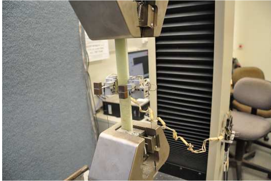
Figure 5.1: Tensile test setup with measurement of longitudinal and transverse strains by a contact extensometer
