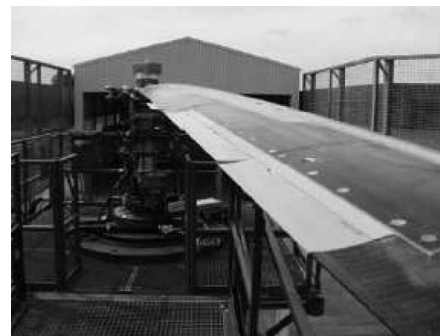
(b) Actively controlled piezoelectric actuated on the BK117 blade (Roth et al. 2006)
