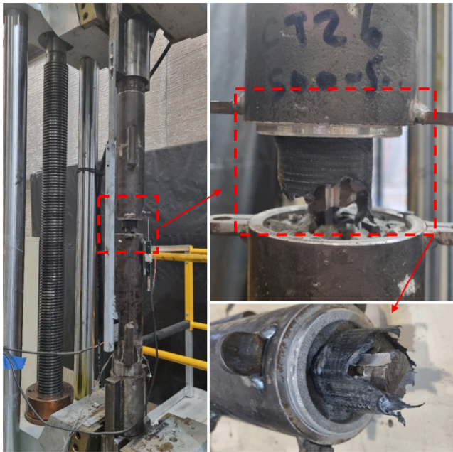
Fig. 16. The conditions of specimen C after testing.
