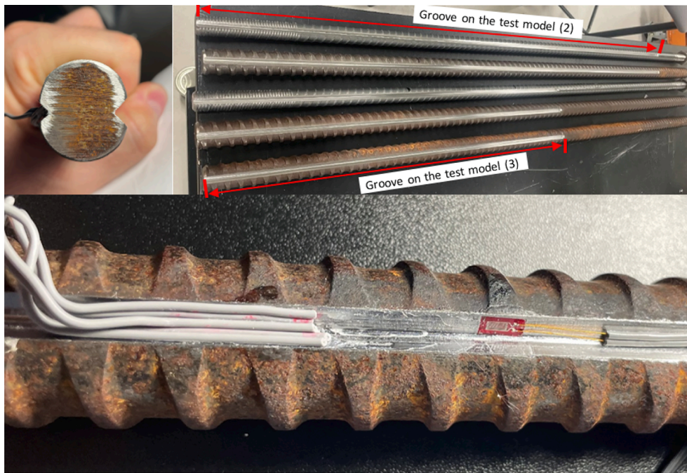
Fig. 7. Grooves, instrumentation, and mounting strain gauges on the steel bars.
