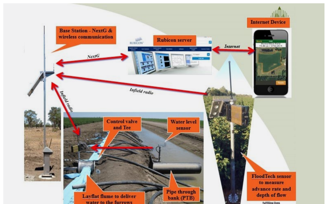
FIGURE 1. Automated furrow irrigation tested in field.
