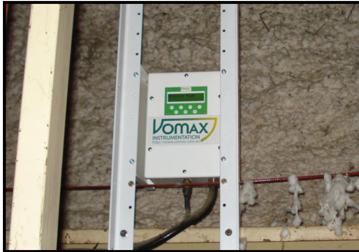
Figure 6.1: Microwave moisture sensor located at gin feeder bay
