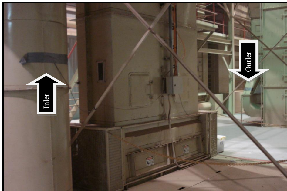
Figure 6.9: Temperature probes were inserted to drilled inlet and outlet air pipes
