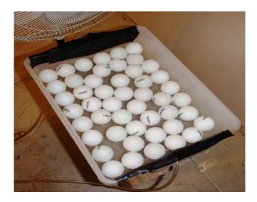
Figure 3: Ping pong balls in formation across the small water tank used in the experiments.
