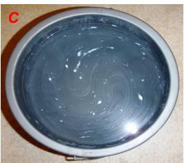
**Figure 1:** A) WaterSavr chemical film unevenly spread out over a water surface. B) Aquatain chemical film randomly distributed over a water surface. C) Octadecanol monolayer spread on top of a water surface.
