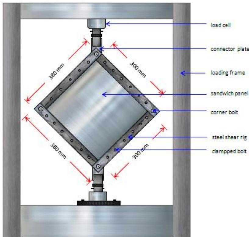
Figure 7.7. Schematic illustration of diagonal tension shear test
