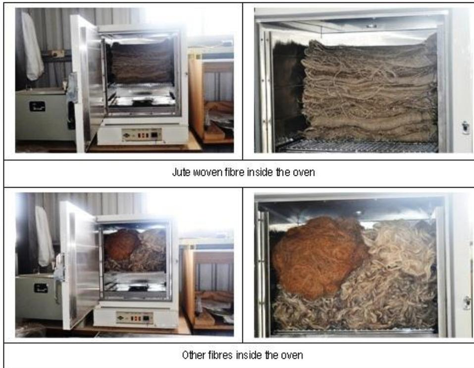
Figure 4.4. Final drying of natural fibres
