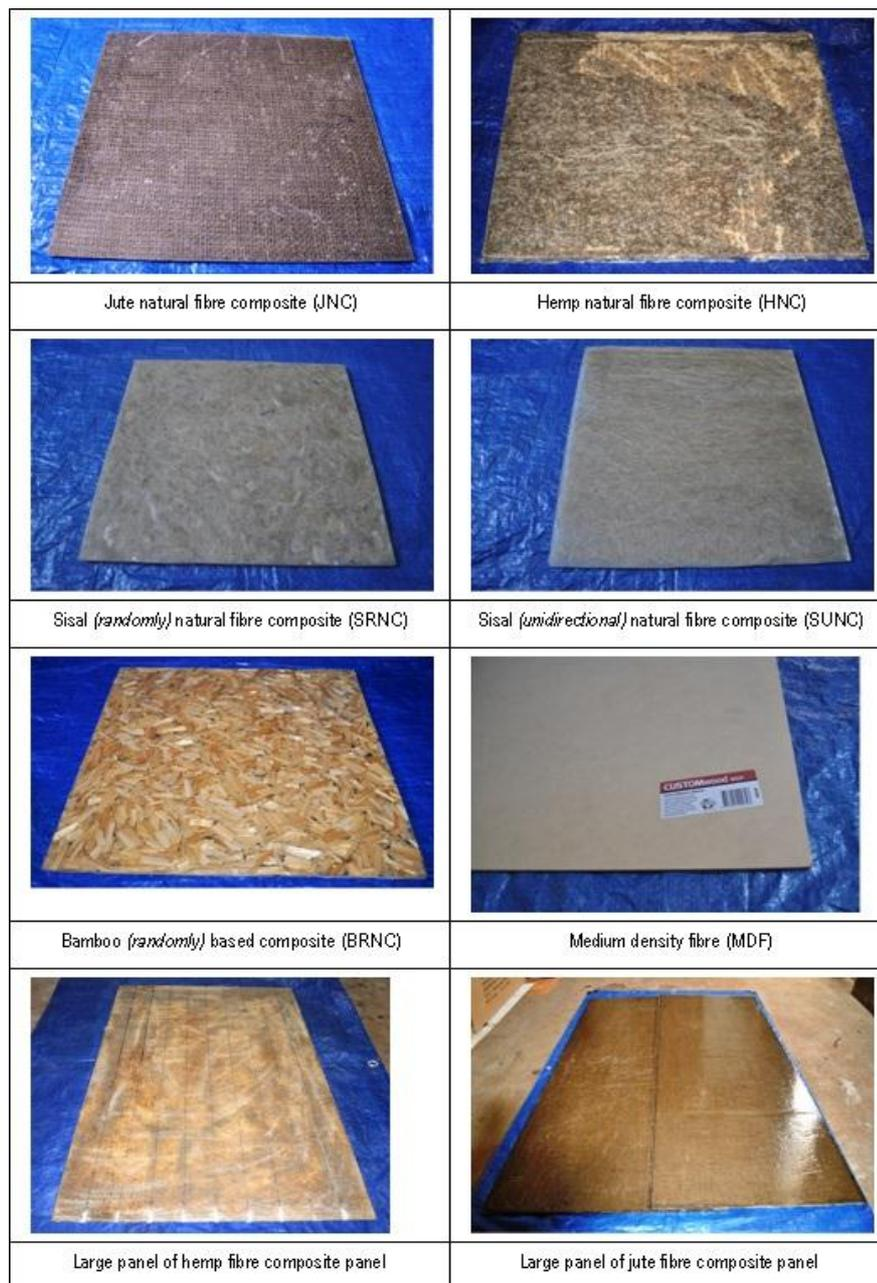
Figure 4.9. Natural fibre based panels and MDF panel prepared for mechanical characterization testing
