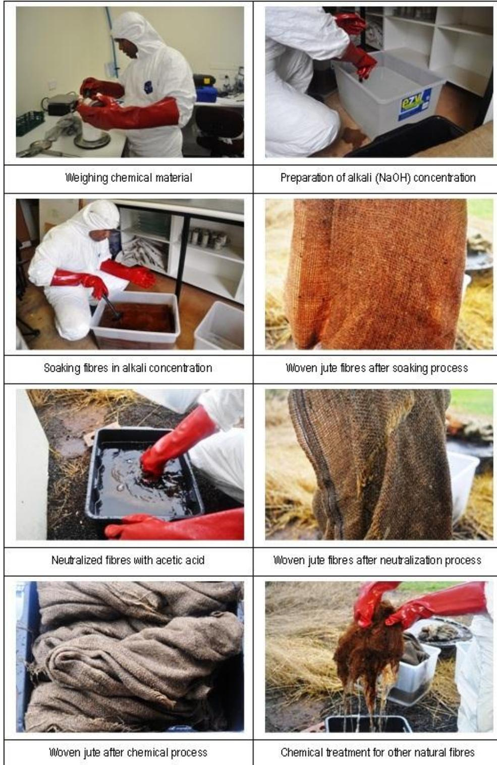
Figure 4.3. Step-by step of alkali treatment of natural fibres
