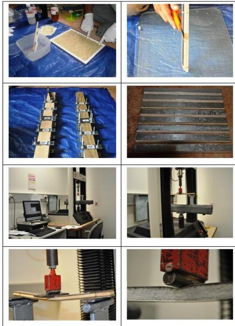
Figure 3.13. Specimen preparation and flexural testing
