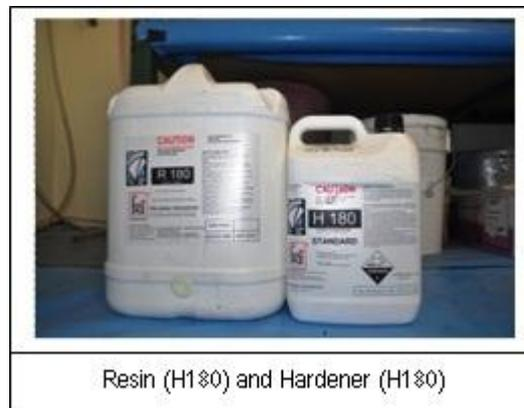
Figure 4.5. The combination of resin and hardener system used in this research
