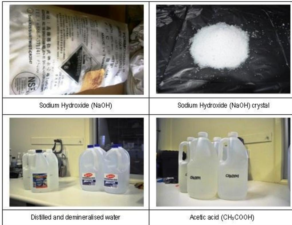
Figure 4.2. Chemicals used for the alkali treatment of natural fibres
