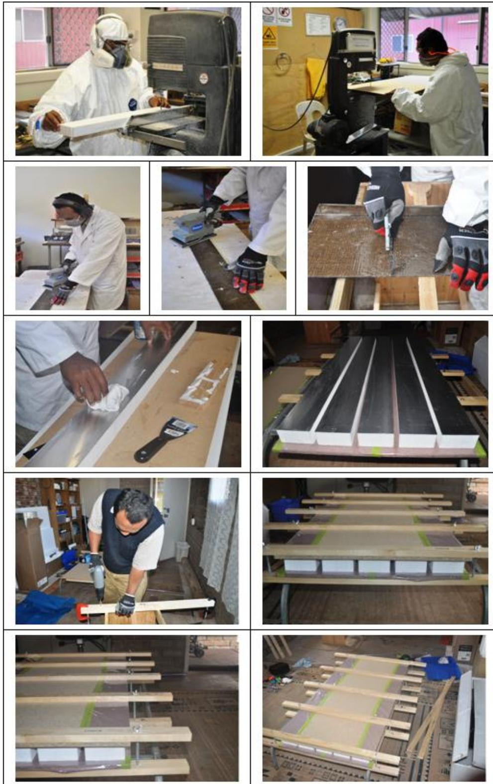
Figure 5.1. Sandwich panel fabrication process
