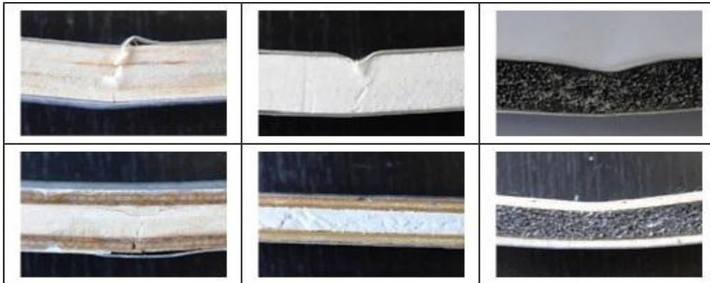
Figure 3.12. Typical failure patterns of unmodified sandwich panel (*above*) and modified sandwich panel (*bottom*)
