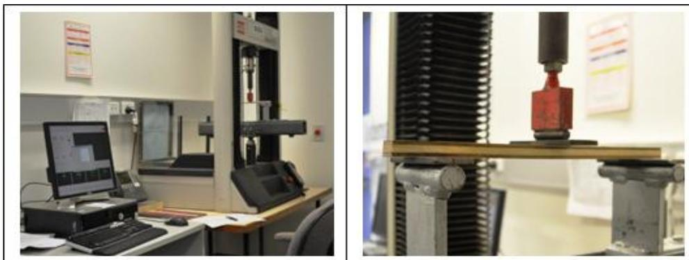
Figure 3.9. *Left*: MTS Alliance RT/10 testing machine connected to computer device. *Right*: Sample set-up under three-point bending loads scheme.
