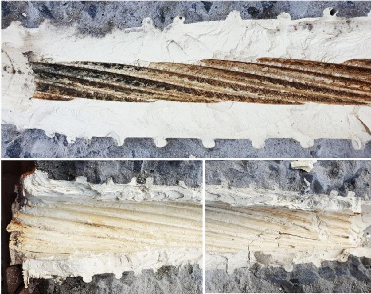
*Figure 16 Top: Indentation imprints of IDSuperstrand cable, Bottom: Broken sample 12S. Dull top and sharp bottom (below the bulb): Left = Collar, Right = Bulb*
