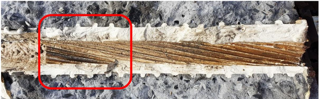
*Figure 17 Broken Goliath cyclic sample - sharper ridges in the bottom and duller towards the collar*
