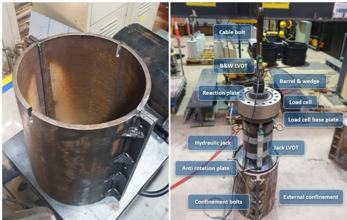
Figure 7 Left: External confinement, and right: Instrumentation and testing components
