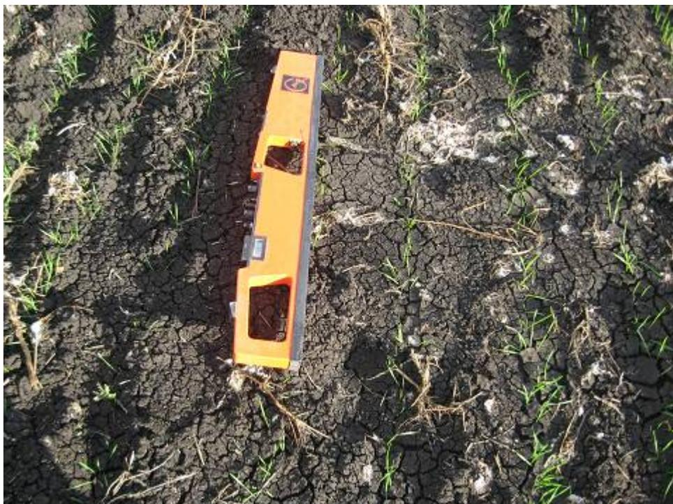
**Figure 2.** Operation of EM38 in horizontal mode (HM) at the soil surface in the wheat field.
