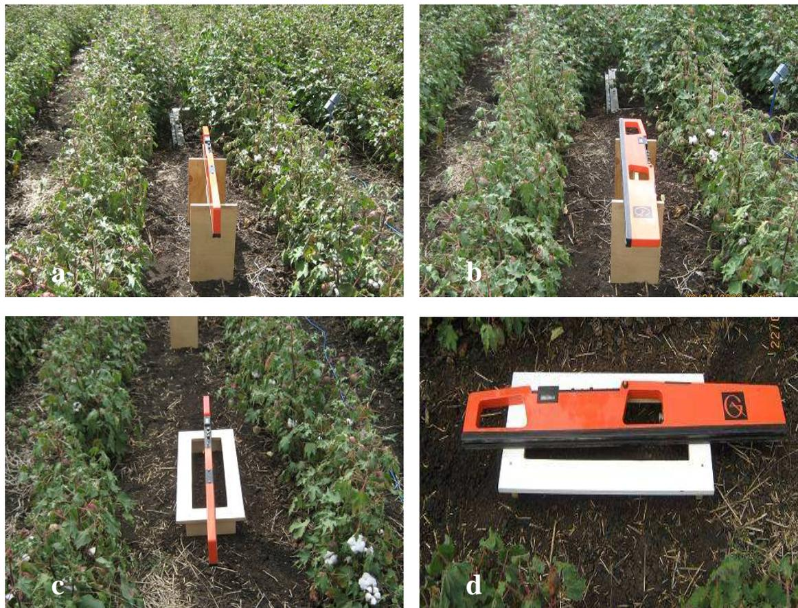
Figure 3. EM38 measurements at various heights above the ground shown for a cotton field. (a) VM – 0.4 m height, (b) HM – 0.4 m, (c) VM – 0.1 m and (d) HM – 0.1 m.
