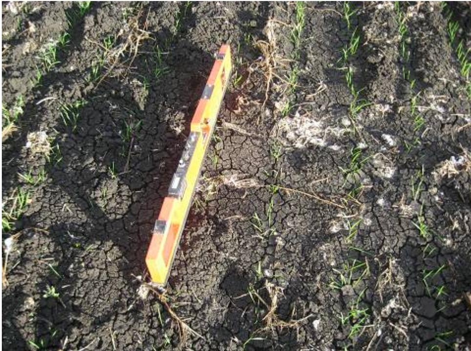
**Figure 1.** Operation of EM38 in vertical mode (VM) at the soil surface in the wheat field.
