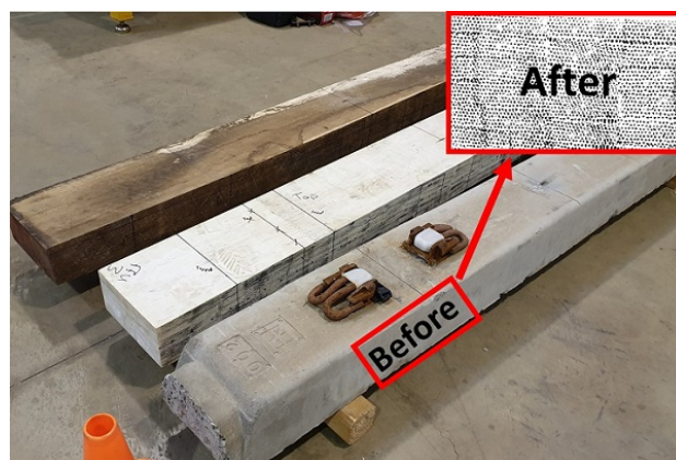
Figure 6. Sleeper samples showing applied speckle pattern.
