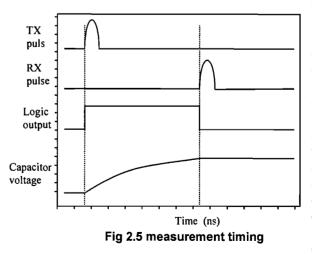
The capacitor in this configuration has а nonlinear charge characteristic which is compensated for in the software. This has the effect of giving a higher resolution at shorter distances and courser at the longer ranges. The charging circuit time constant is approximately 400ns. To clear the timing capacitor the ADC input pin is changed to an output and set low.
