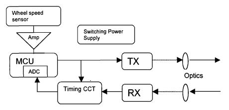
Fig 2.3 System block diagram
