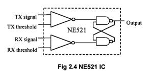
feeding a configurable nand gate flip flop. A TX pulse will set the flip flop and arrival of the RX pulse will cause it to reset. While the flip flop is enabled, a capacitor will charge up to a voltage proportional to the time period and measured range. Figure 2.5 shows a timing diagram of these events.
