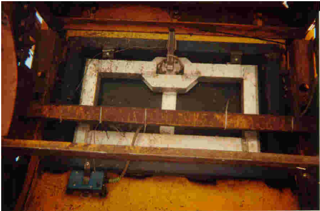
Figure 7-22. The weigh pad installed in the harvester (viewed from underneath the elevator)
