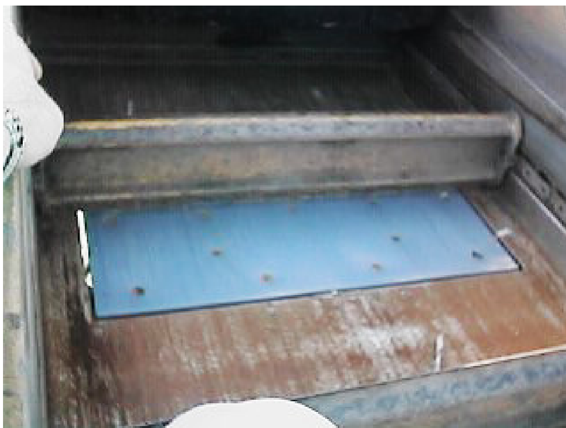
Figure 9-4. Topside view of weigh pad installed in a Cameco harvester.
