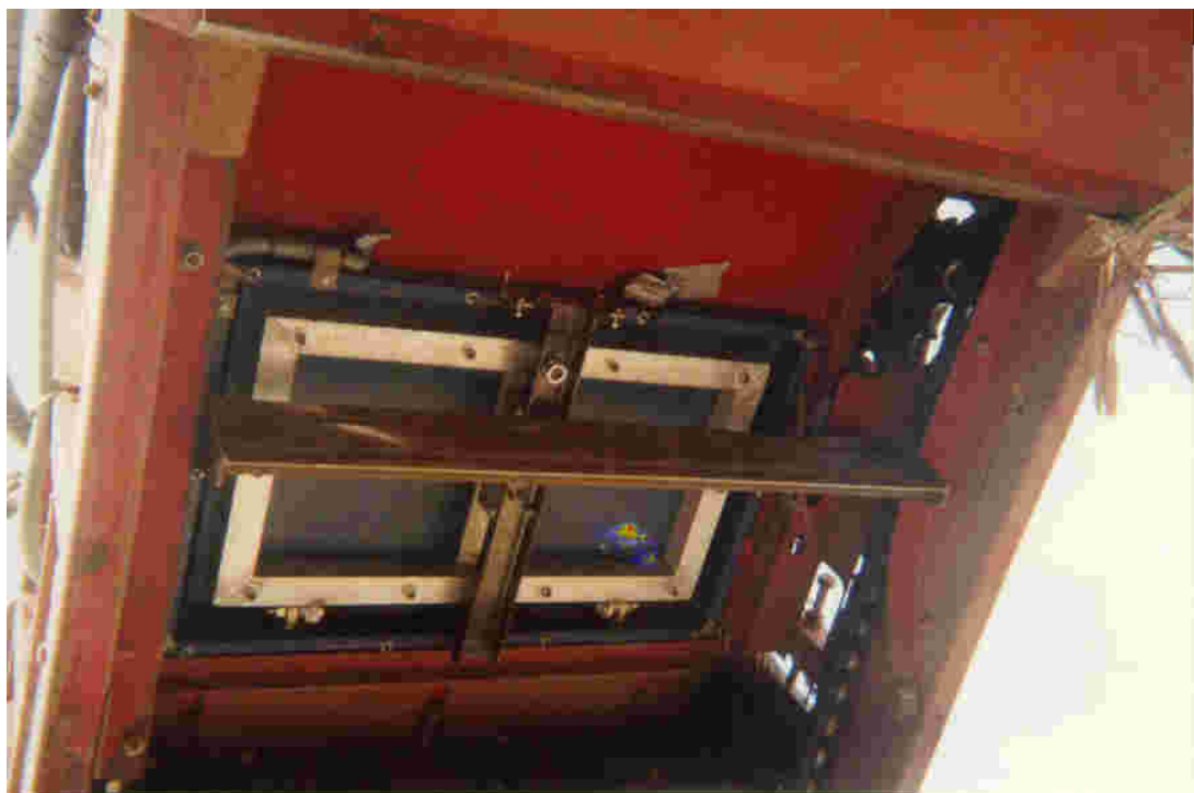
Figure 9-3. Underside view of weigh pad installed in an Austoft harvester.
