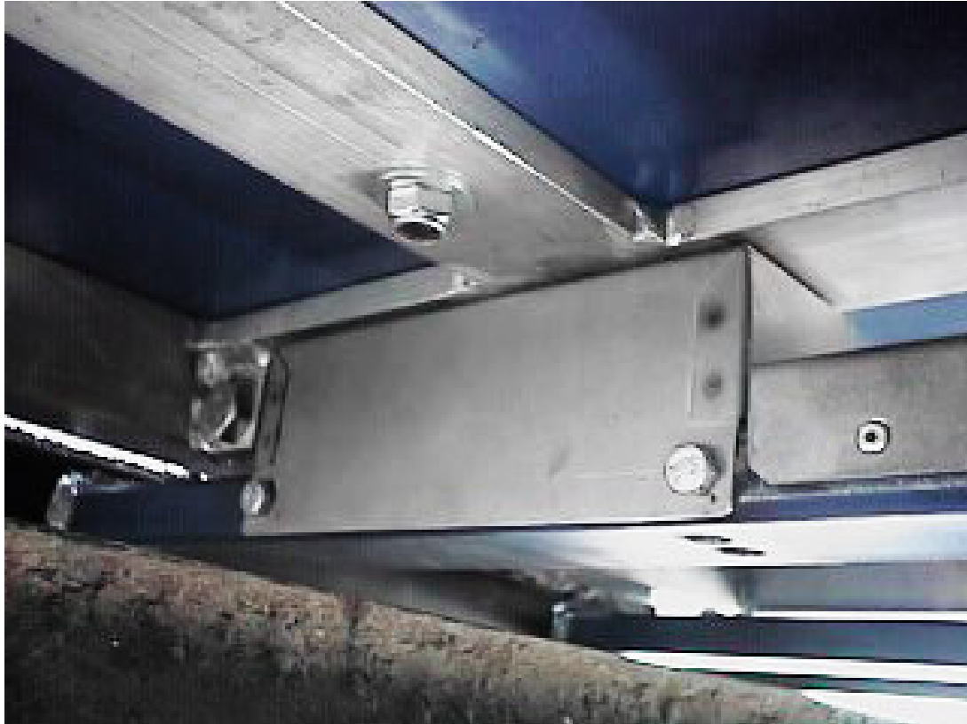
Figure 9-5. Close-up view of the load cell mount assembly installed on a Cameco harvester.
