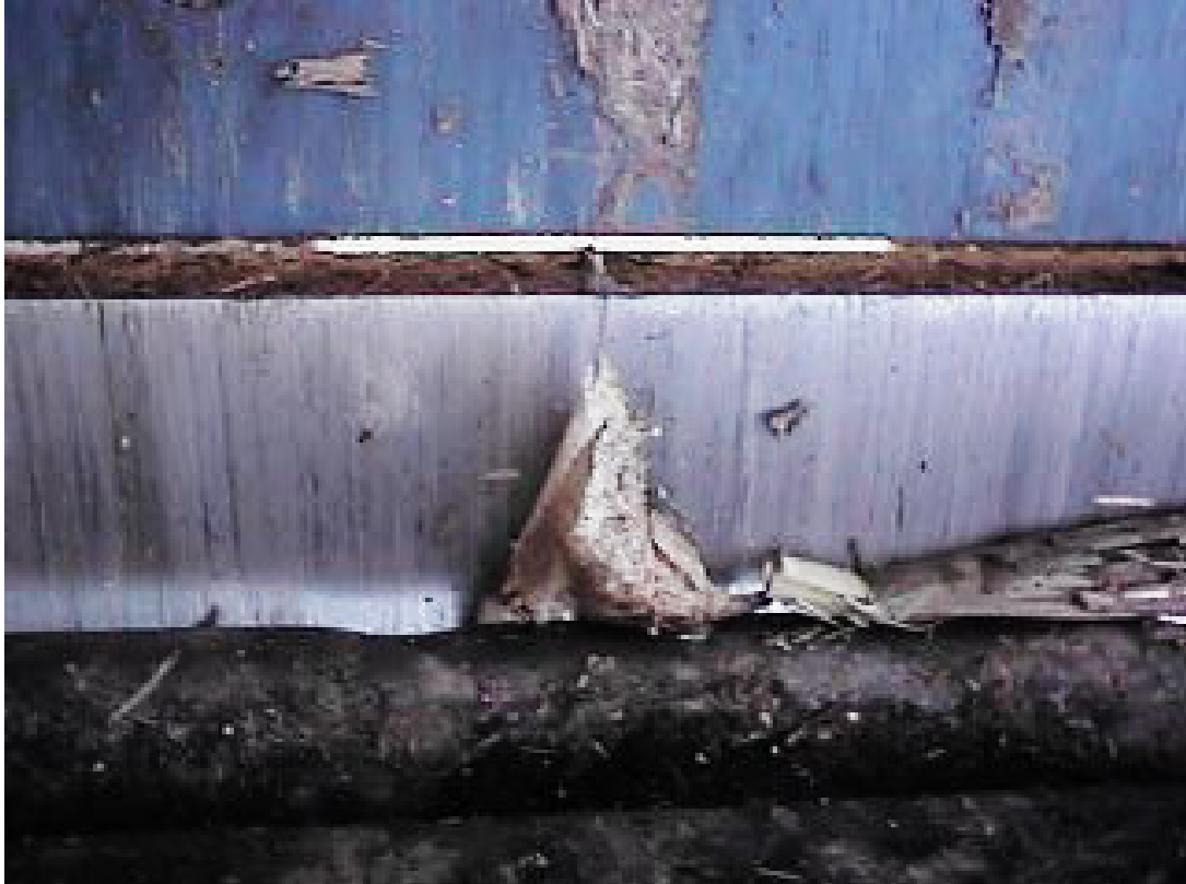
Figure 10-9. Piece of sugar cane billet wedged under an elevator flight just prior to travelling over the weigh plate. (Viewed from in front of the flight).
