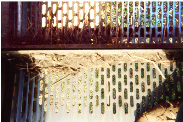
Figure 10-8. Build up of extraneous matter (mud and leaf matter) on the base of an elevator flight. (Viewed from above the flight).
