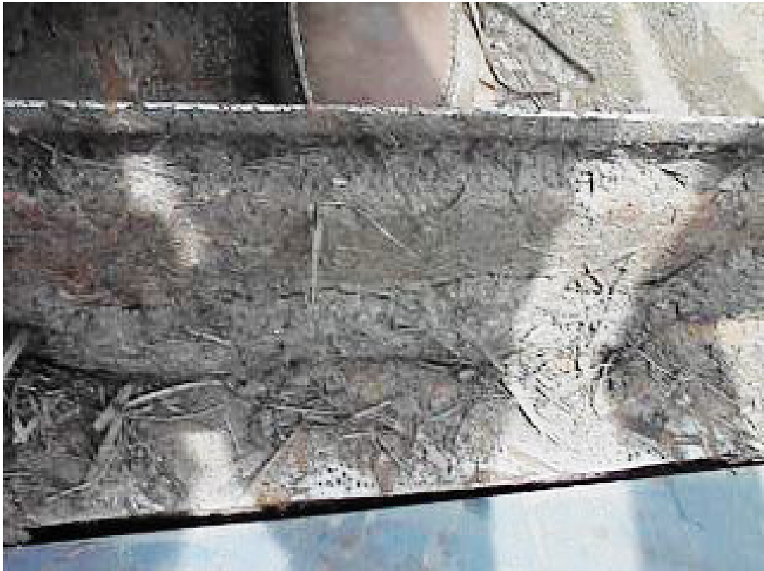
Figure 10-7. Build up of extraneous matter (mainly mud) on the base of an elevator flight just prior to travelling over the weigh plate. (Viewed from above and in front of the flight).
