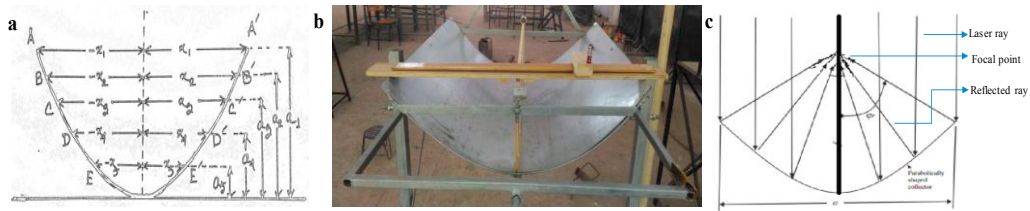
Fig. 5. Profile error measurement (a) depth of parabola at different test point; (b) experimental setup; (c) theoretical background of slope error measurement.
