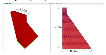
Figure 1. The FE model of the concrete dam block structure
