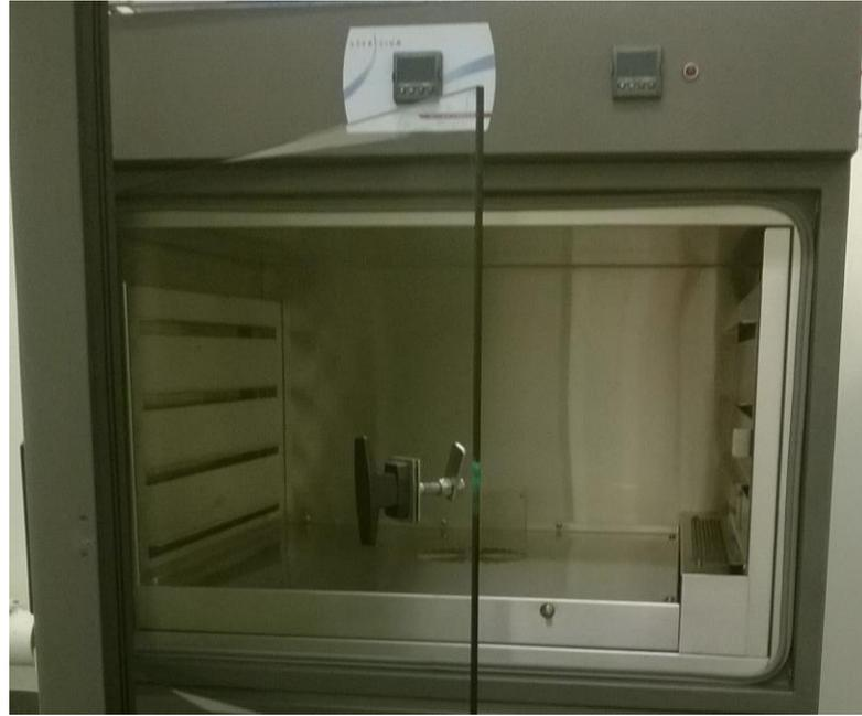
**Figure 4-2. The Steridium Environmental chamber used to control temperature and relative humidity to allow the determination of thin layer drying rates (load cells were placed on shelves inside the chamber).**
