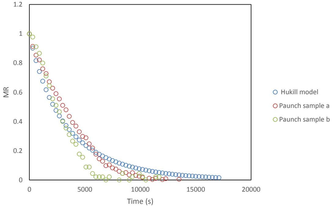
**Figure 9-6. A non-linear regression was used to find the optimum  $D$  value for the set conditions, this gave  $D = -0.714$  in the Hukill equation producing an  $R^2$  of 0.928.**
