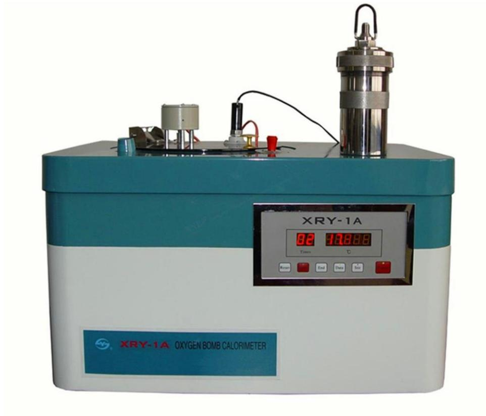
**Figure 6-1. An XRY-1A Oxygen Bomb Calorimeter (Nanbei 2014).**
