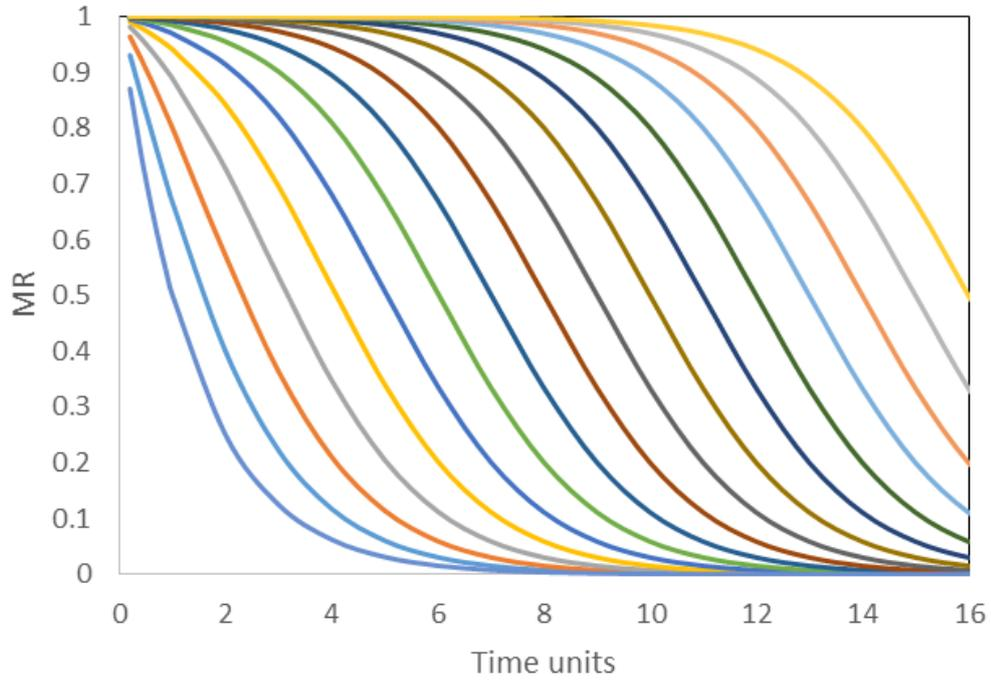
**Figure 9-1. The standard deep bed drying curves from the Hukill equation.**
