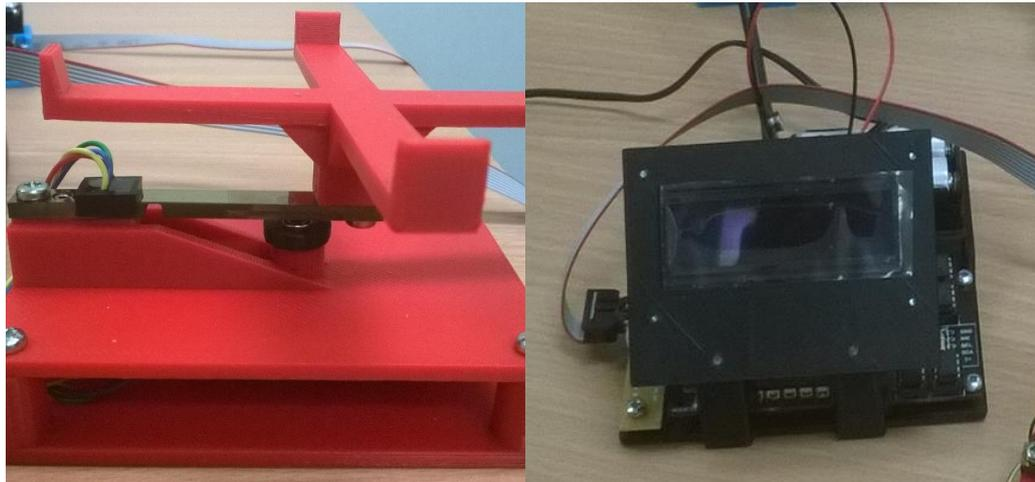
**Figure 4-1. A 50 gram load cell and tray holder (left) wired into a custom built data logger (using a Picaxe microcontroller) (right).**
