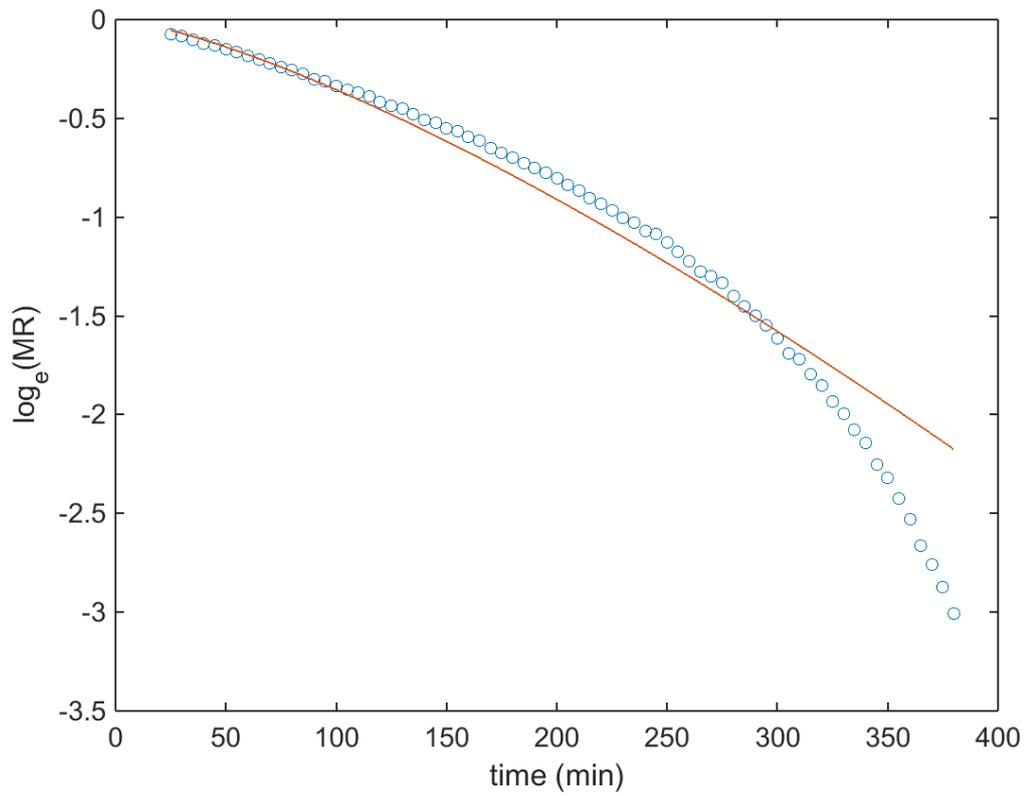
**Figure 4-9. Page equation fit for 35 °C, 50% relative humidity thin layer grass type sample.**
