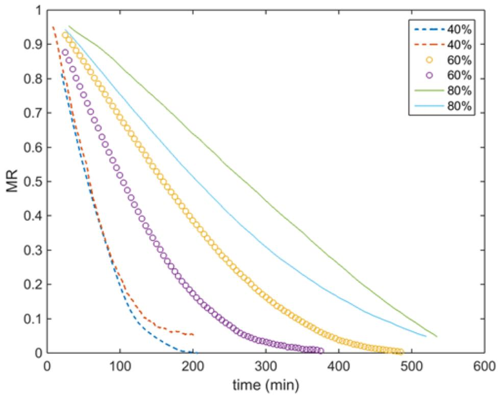
**Figure 4-5. The MR over time (min) for 35 °C air at 40, 60, and 80% RH.**
