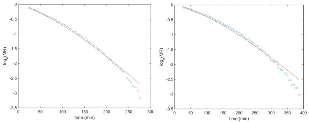
**Figure 4-10. Page equation fit for 35 °C, 60% relative humidity thin layer grain type samples.**
