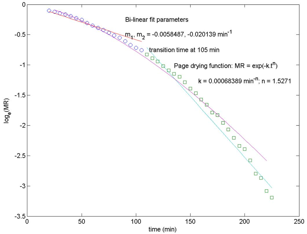
**Figure A-19 - Thin layer grain 55 °C, 50% RH.**
