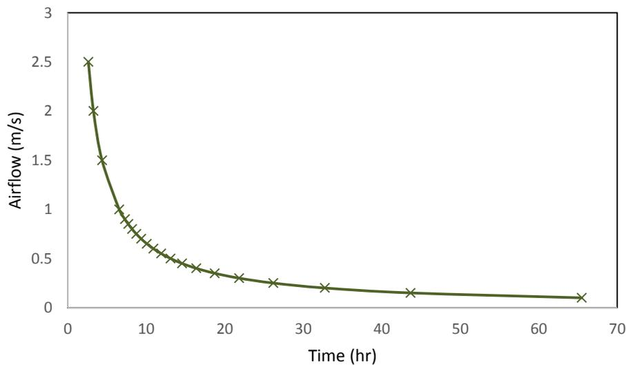
**Figure 8-8-3. Airflow (m/s) versus time (hours). An increase in airflow from approximately 1 m/s does not greatly improve drying rates.**
