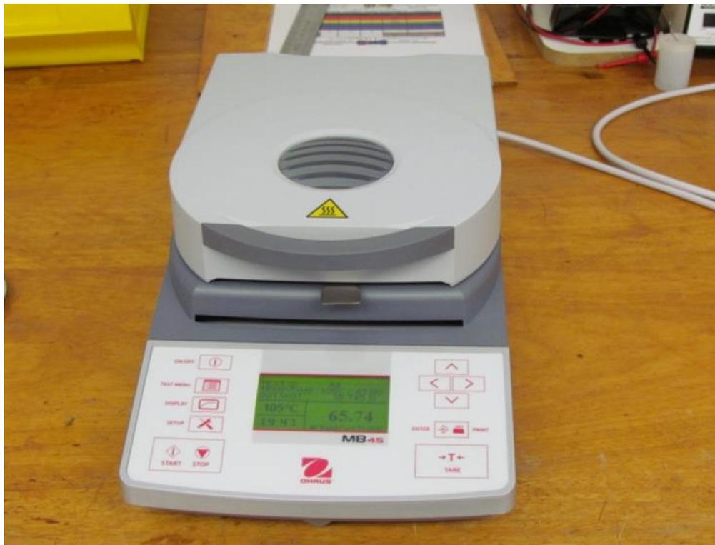
**Figure 3-2. Ohaus MB45 moisture balance used to determine initial, final, and equilibrium moisture content.**
