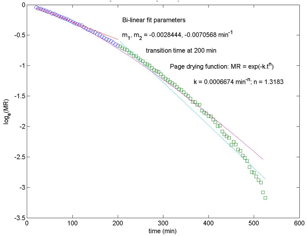
**Figure A-7 - Thin layer grain 35 °C, 80% RH.**
