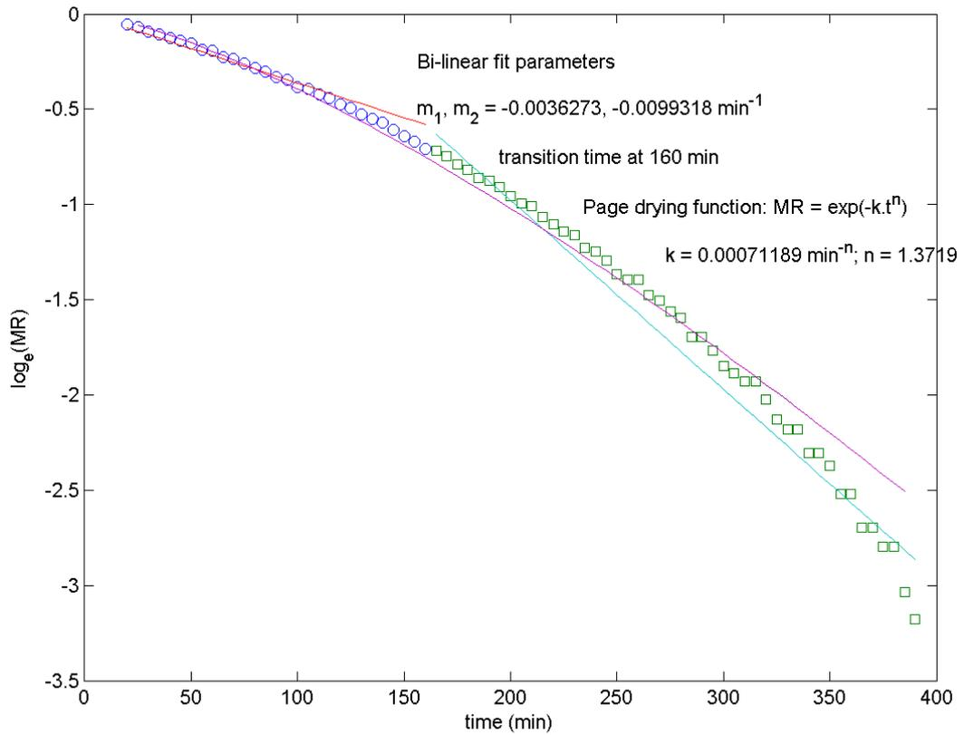
**Figure A-5 - Thin layer grain 35 °C, 60% RH.**
