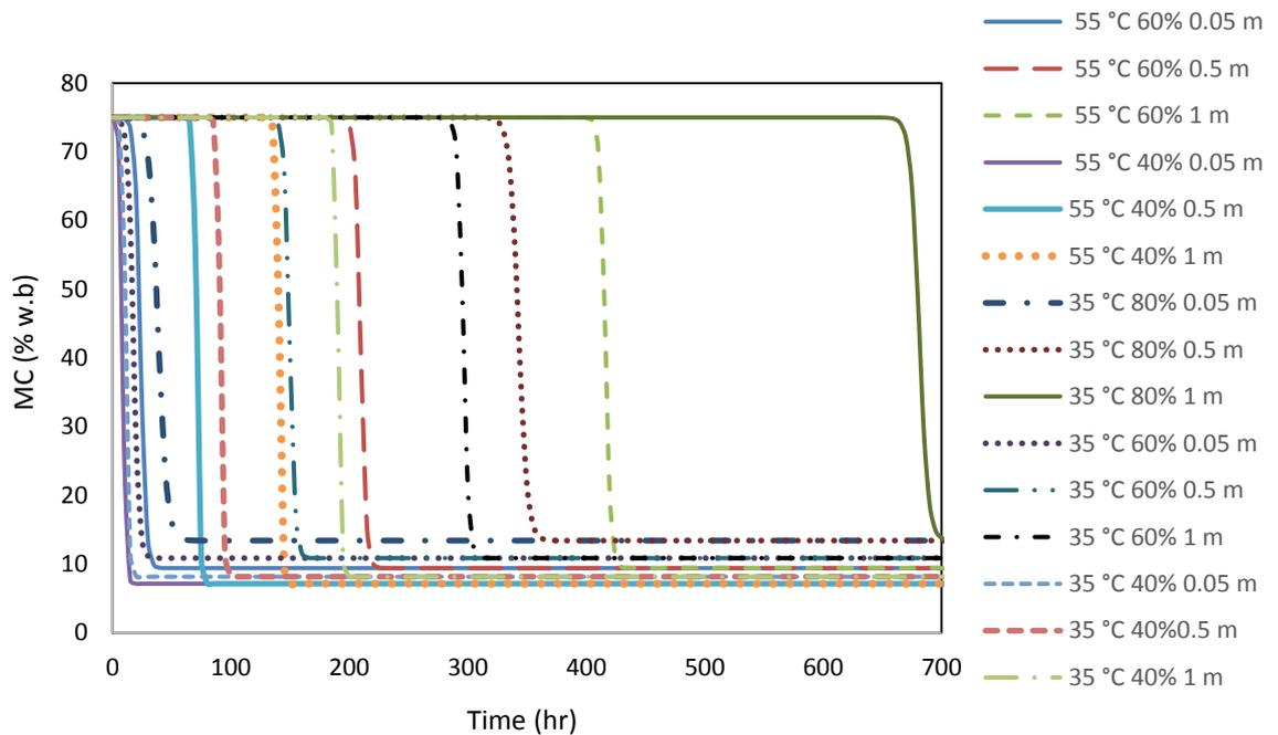
**Figure 9-4. Time for different operating temperatures and depth using the MR half-life values for RH.**
