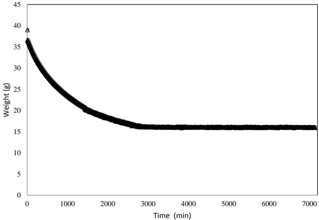
**Figure 4-4. Weight (g) versus time (mins) for 35 °C temperature and 40% relative humidity. The load cell precisely maintained accuracy over time and showed an expected plateau once EMC was met.**
