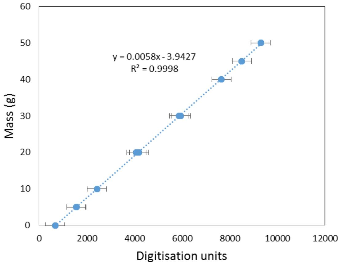
**Figure 4-3. Calibration mass versus digitisation units from the load cell and data logger system.**
