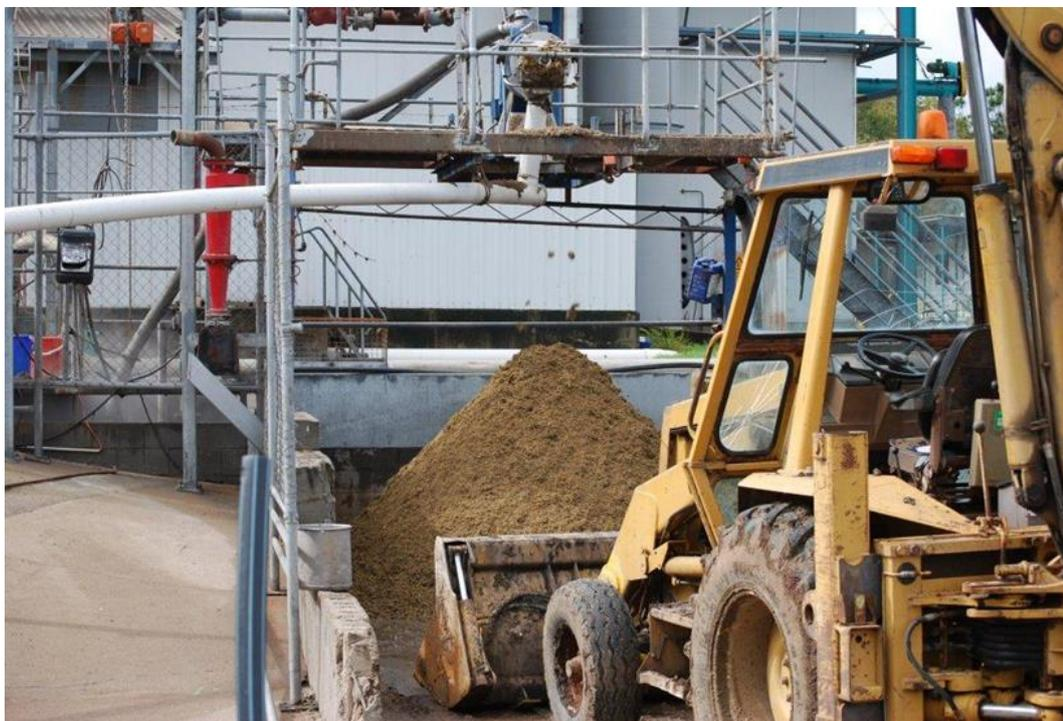
**Figure 2-1. Paunch on site at an Australian RMP plant passes from a screw press to fall into a pile in the cement holding area.**
