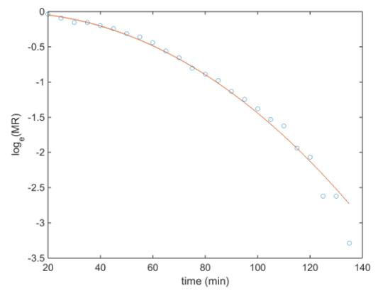
**Figure 4-8. Page equation fit for 35 °C, 40% relative humidity thin layer grain type sample (top) and two grass type samples (bottom).**
