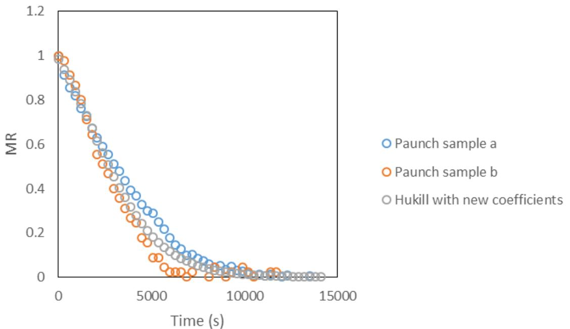
**Figure 9-8. The Hukill equation with coefficients added to the time constant,  $R^2$  values are 0.997 for the thin layer and 0.998 for the 2.5 cm sample.**
