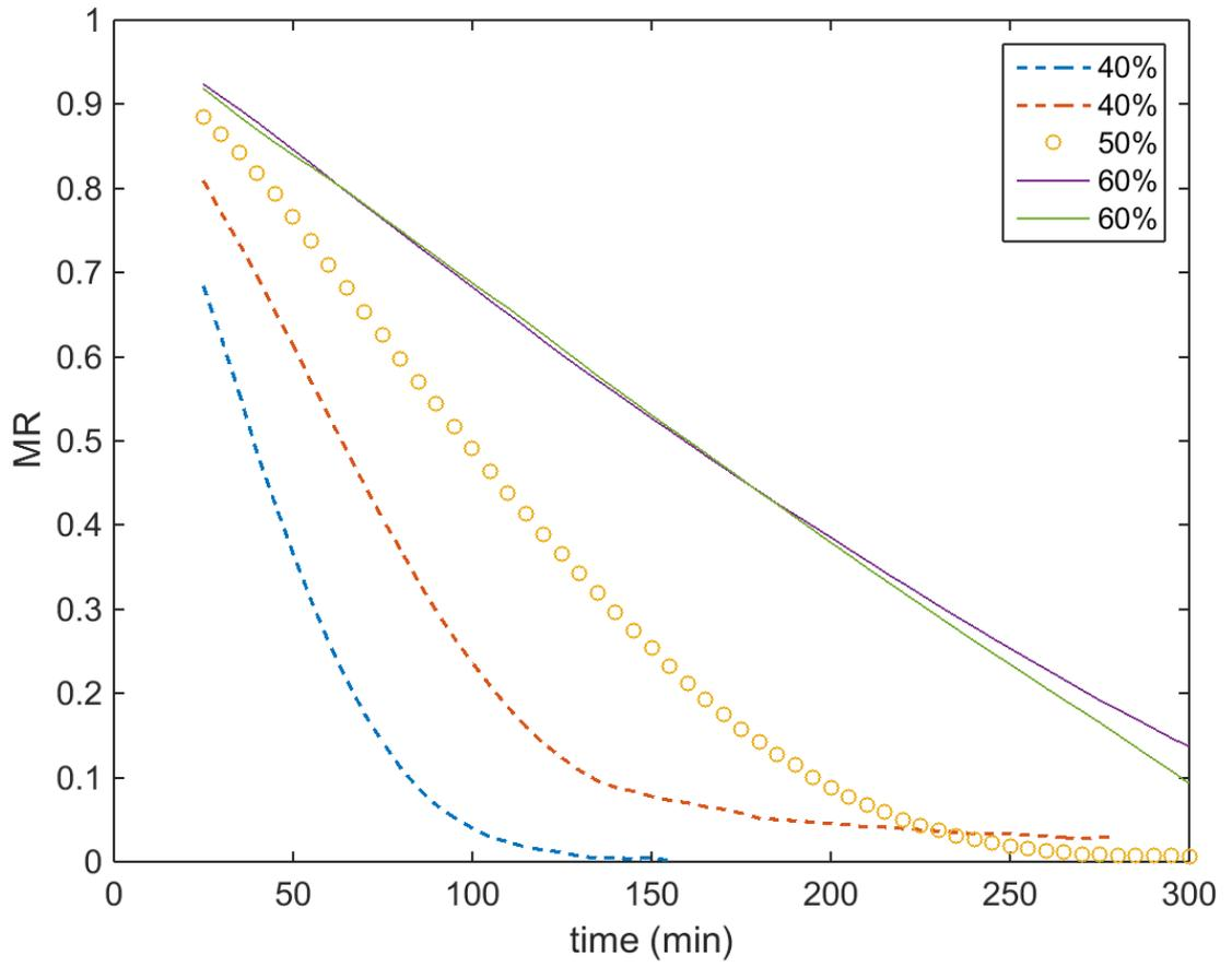
**Figure 4-7. The MR over time (min) for 55 °C air at 40, 50, and 60% RH.**
