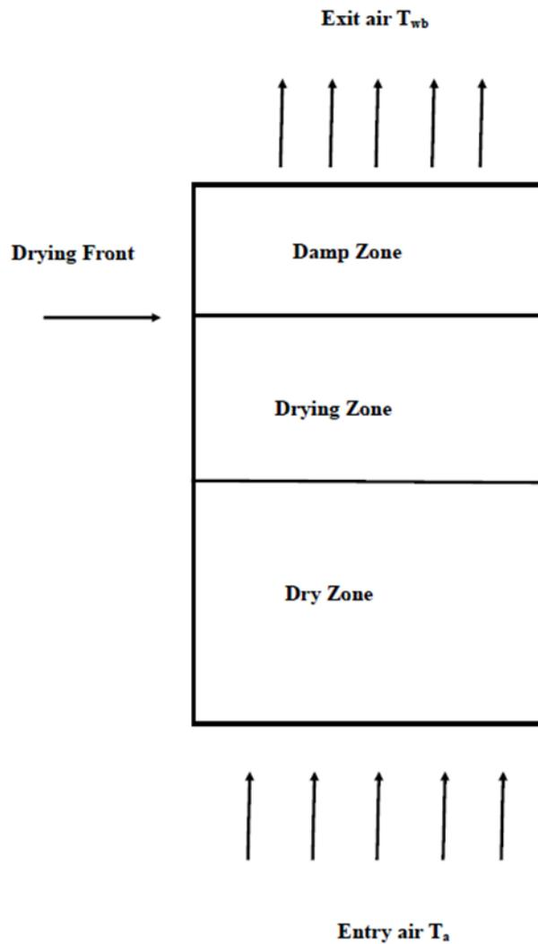
**Figure 8-1. Drying zones produced by the drying front.**
