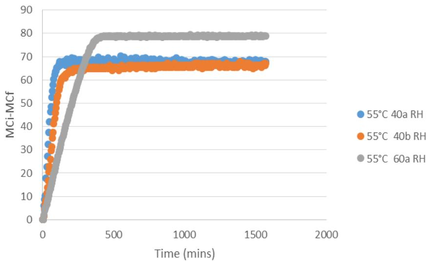
**Figure 7- 55°C air temperature with 40, 60% relative humidity.**
