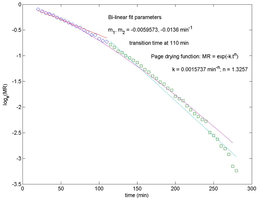
**Figure A-6 - Thin layer grain 35 °C, 60% RH.**
