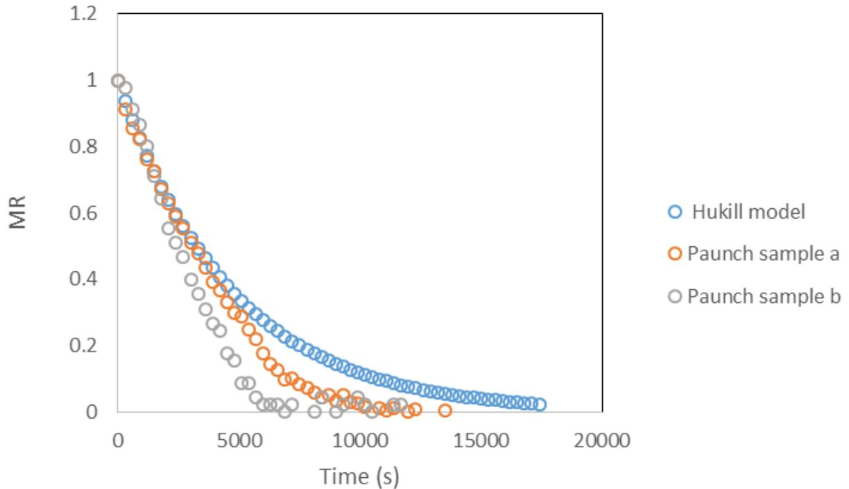
**Figure 9-5. Comparison of Hukill model for  $1 \times 10^{-11}$  m depth to paunch thin layer 35 °C, 40% RH samples a and b.**
