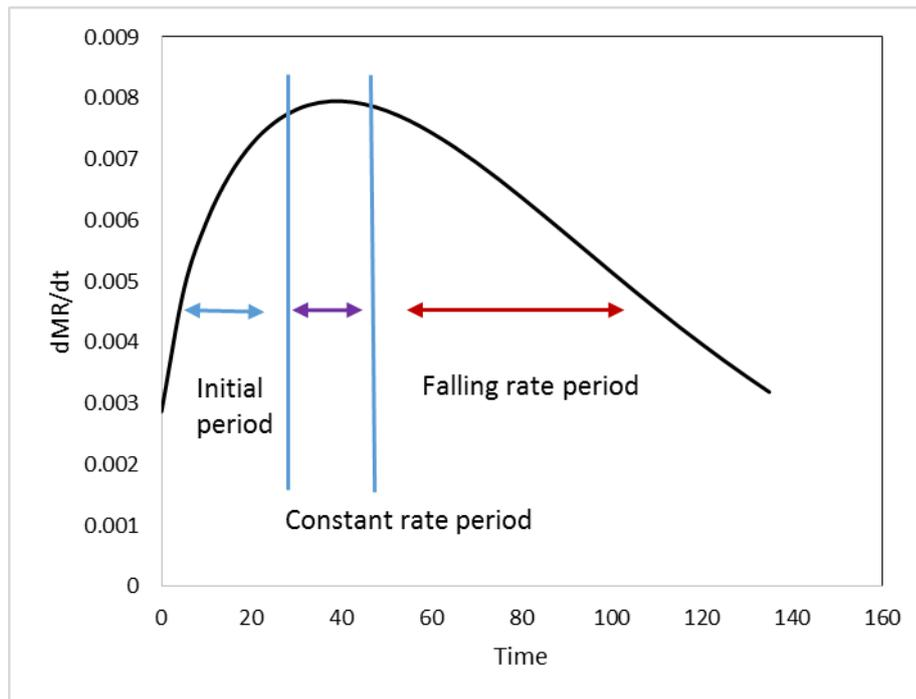
**Figure 4-11. An example of the drying rate versus time graph using the Page equation for 45°C operating temperature shows the expected stages of drying.**
