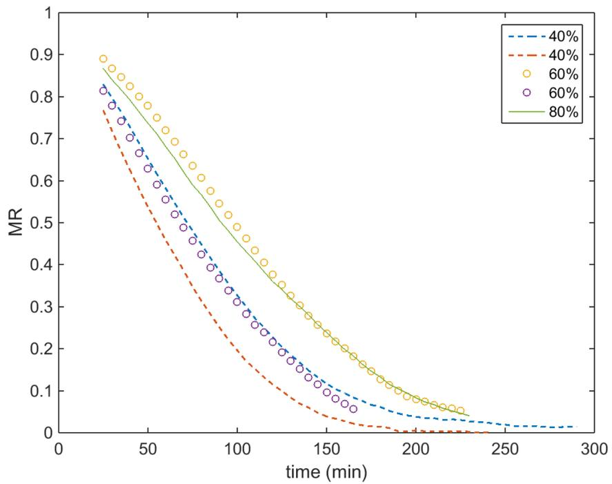
**Figure 4-6. The MR over time (min) for 45 °C air at 40, 60, and 80% RH.**
