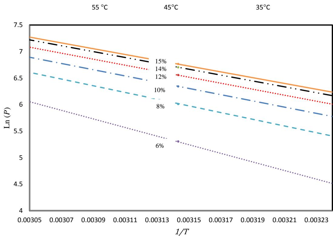
**Figure 5-2. The slope of the natural log of  $P$  versus the reciprocal of  $T$  times the universal gas constant gives the latent heat of vaporisation of paunch.**
