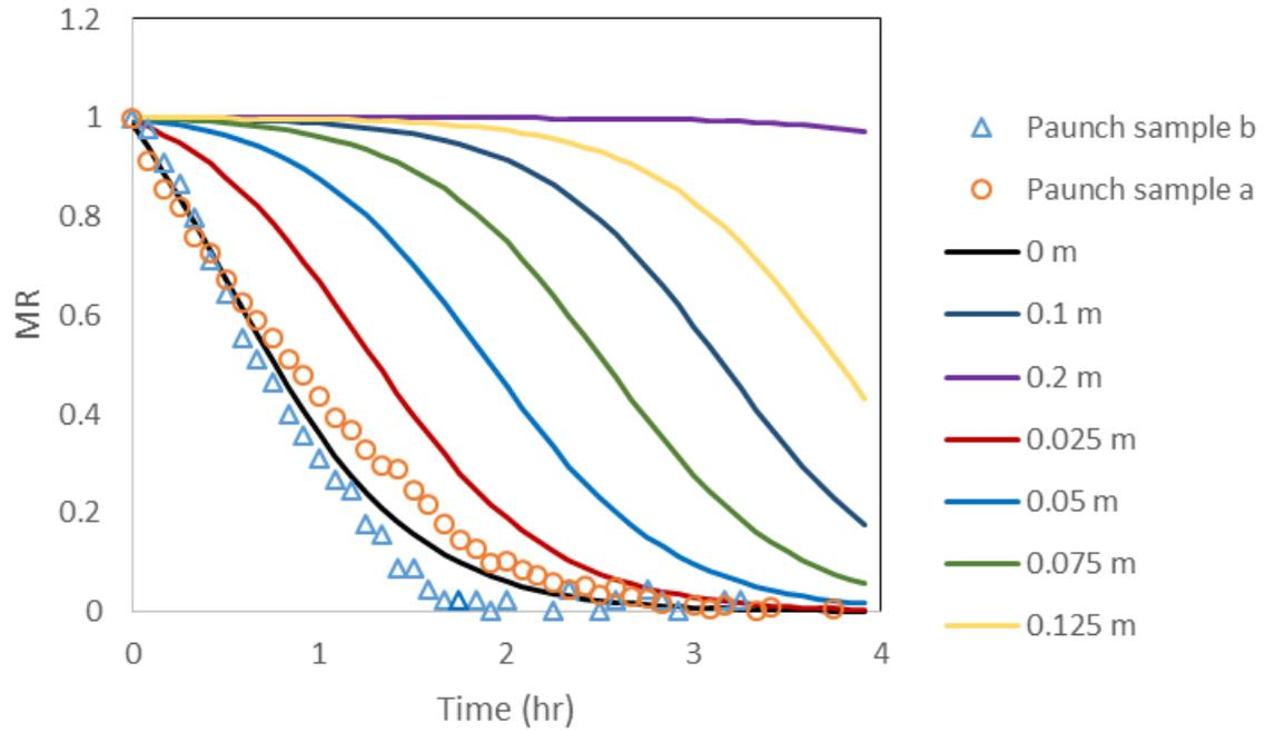
Figure 9-9. Solution to the Hukill equation for paunch at varying depth using new coefficients on the dimensionless time unit.
