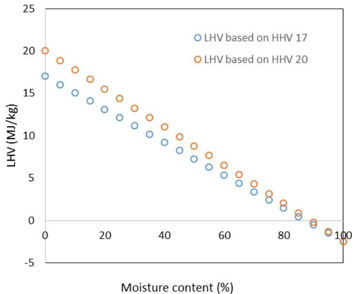
**Figure 6-3. Relationship between moisture content and lower heating value of paunch. As the moisture content increases the calorific value decreases.**
