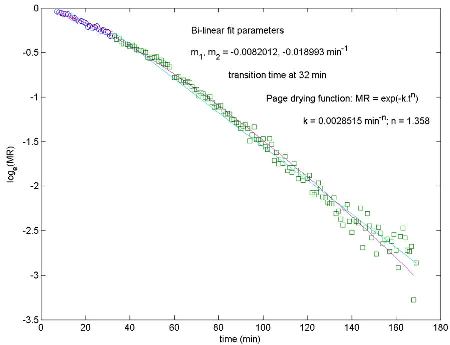
Figure A-1 - Thin layer grain 35 °C, 40% RH.
