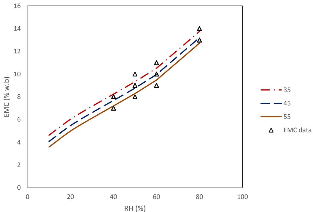
**Figure 5-1. Desorption moisture equilibrium isotherms predicted for 35, 45, and 55 °C using Chung-Pfost equation with acquired data for 40, 50, 60, 80% RH (EMC data points indicated above are average values for EMC to allow visual comparison to model).**
