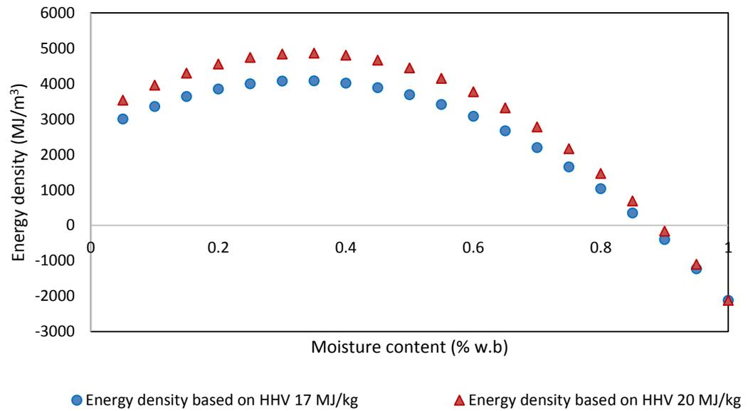
**Figure 7-1. Graphical representation of energy density versus moisture content.**
