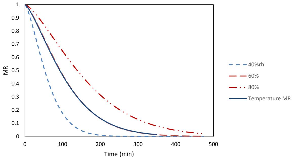
**Figure 9-3. MR versus time (min) for MR (40, 60, 80% RH) and MR (35, 45, 55°C).**
