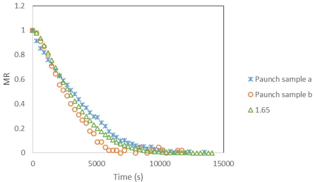
**Figure 9-7. A plot of the experimentally determined thin layer constants applied to the constants in the 2<sup>nd</sup> and time based Hukill equation with the experimentally determined thin layer paunch samples.**
