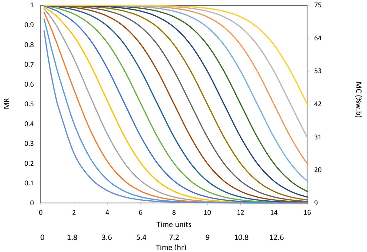
**Figure 9-2. Example drying curves for the Hukill equation using the thin layer half-life,  $t_{MR(0.5)}$ , for 40% RH with 0–16 depth units. Each time unit is 0.9 hours with an initial MC of 75% (w.b).**
