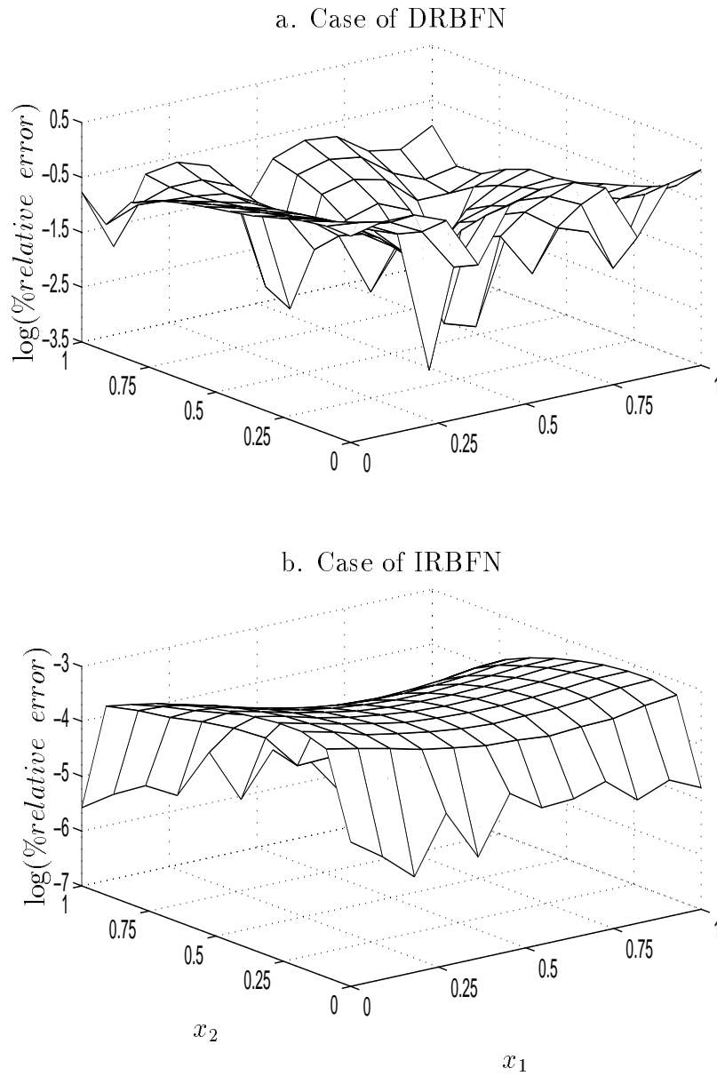
Figure 16: Error in the solution of \nabla^2 u = (\lambda^2 + \mu^2) \exp(\lambda x_1 + \mu x_2) : the numerical solutions are obtained with \beta = 8 in both DRBFN and IRBFN methods. Percentage relative error is used in the plot. For the IRBFN, the error distribution is seen to be smoother and particularly the error is smaller along the boundary in comparison with the case of DRBFN.
