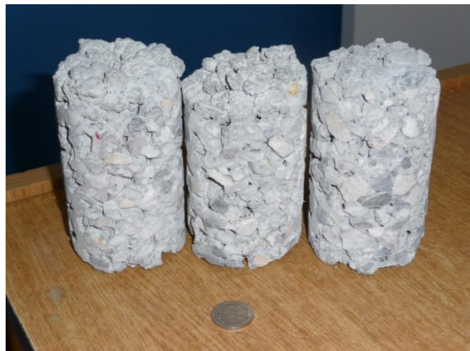
Figure 4.6 75mm Concrete Cores
