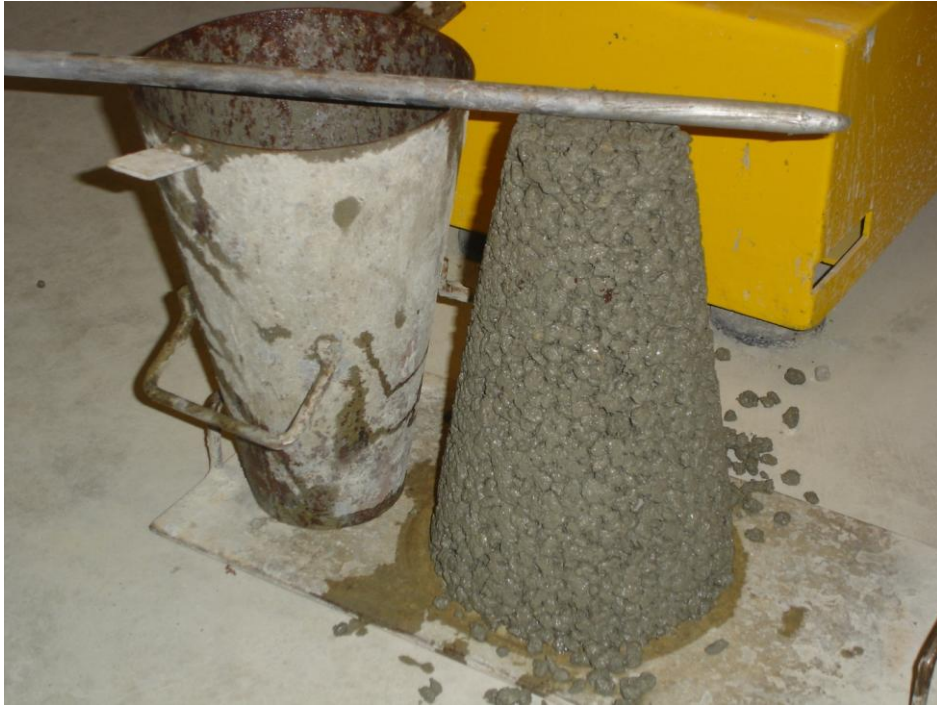
Figure 4.3 Slump Testing on a Trial Mix
