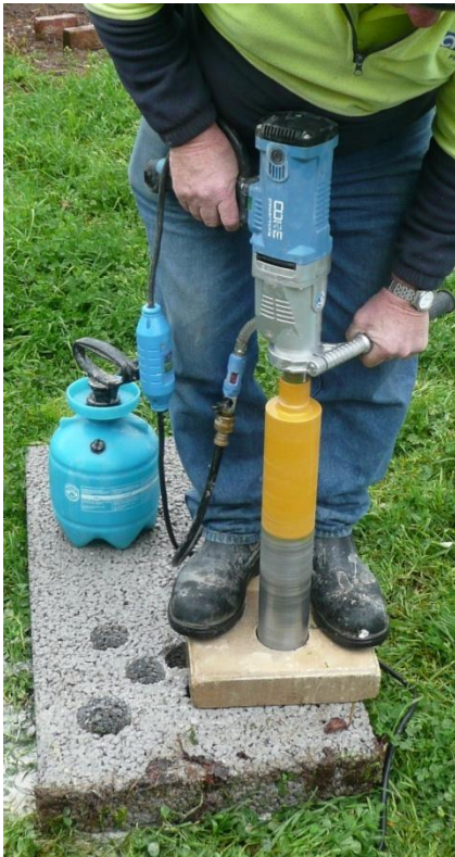
Figure 4.5 75mm Cores Being Cut From Cast Concrete Sample.
