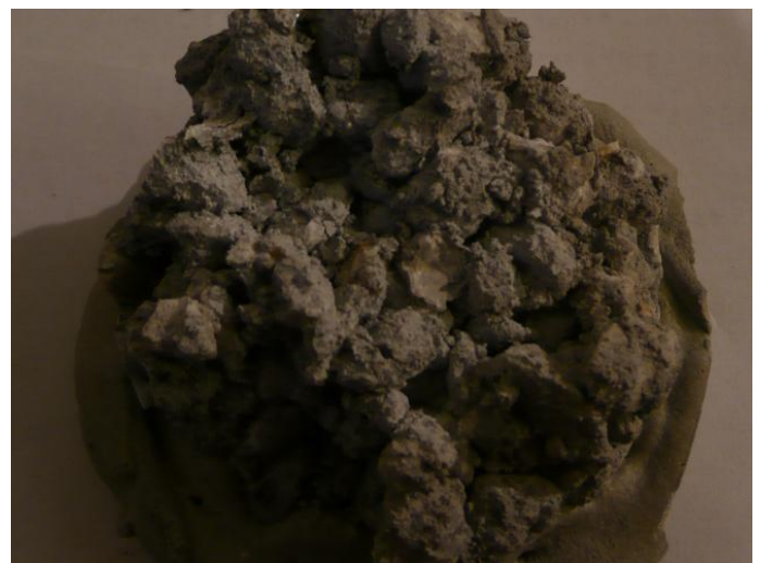
b) Trial 7, 30% void ratio, 10% \text{TiO}_2
