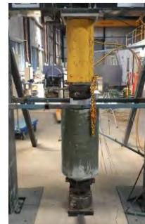
Figure 1. Test set-up for columns
