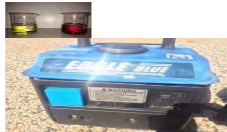
Figure 1 electrical generator operated with waste cooking oil and petrol.
