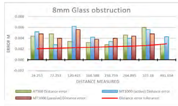
Figure 1: 8 mm Glass obstruction distance errors
