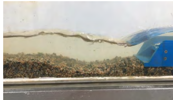
Figure 1 – Culvert scouring under high velocity conditions
