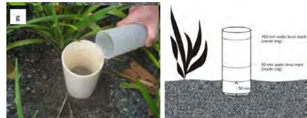
Figure 1 – Single ring infiltrometer test procedure (FAWB 2009)
