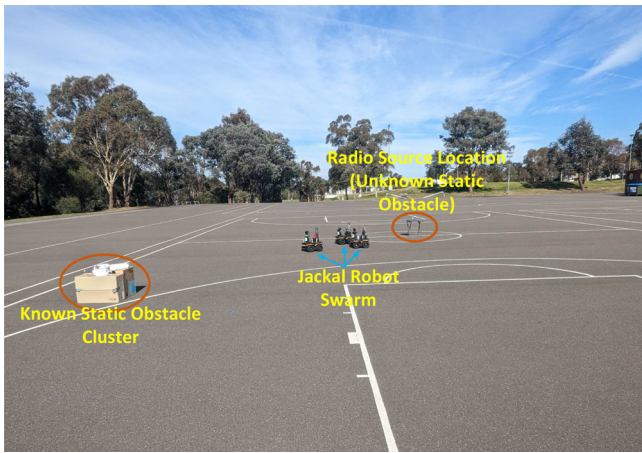
FIGURE 6 | Experimental setup. The radio source is placed close to the middle of the mapped area, and its location is measured using a GPS sensor. [Color figure can be viewed at wileyonlinelibrary.com ]
