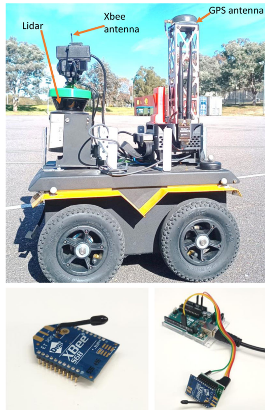
FIGURE 8 | The Jackal mobile robot used for the radio source localization and field tests is shown on top. The XBee modems are mounted on the robot with the help of a plastic bracket. The XBees are placed as high as possible on the robot to minimize ground reflections. The XBee modem and the Arduino attachment used for the testing are shown at the bottom. [Color figure can be viewed at wileyonlinelibrary.com ]
