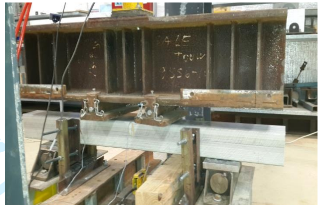
Figure 1. Experimental set-up for characterisation of elastic properties
