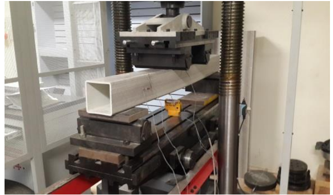
Figure 1. Experimental set-up for characterisation of elastic properties
