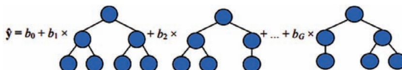
Figure 2. Multigene symbolic regression. The prediction of the response data y is the vector output of G trees modified by bias term b_0 and scaling parameters b_1, \dots, b_G .
