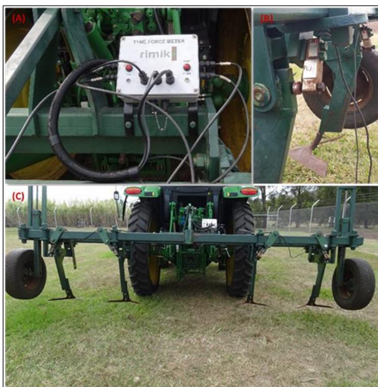
**Figure 3.3: Overview of the experimental tillage unit used in the study; (A): Close-up of data-logger, (B): Close-up of force transducer; and (C): Plan view of tractor and tillage unit**
