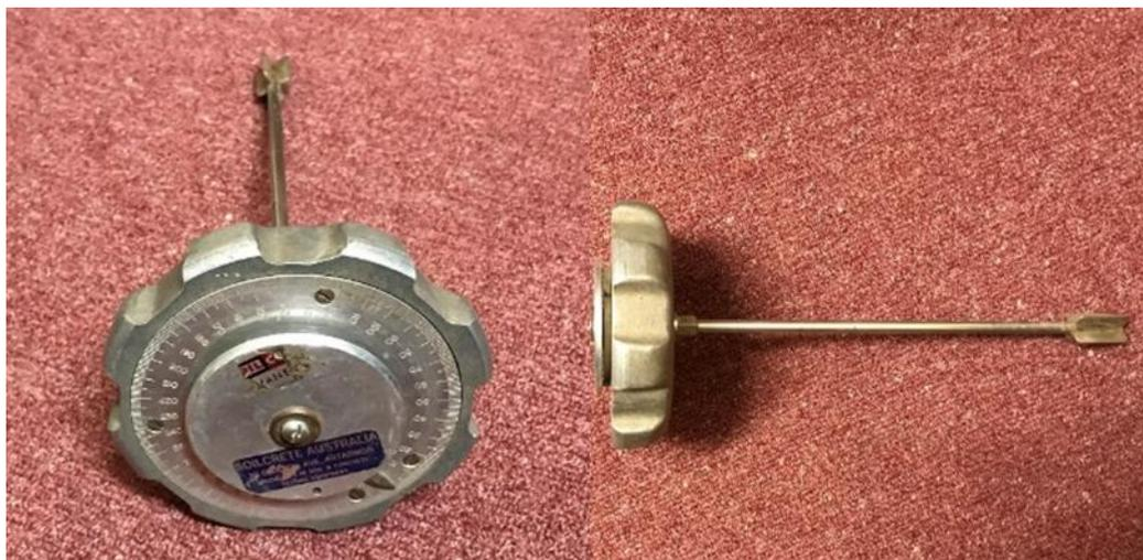
Figure A3.3: Shear vane used to measure shear force of studied soils.
