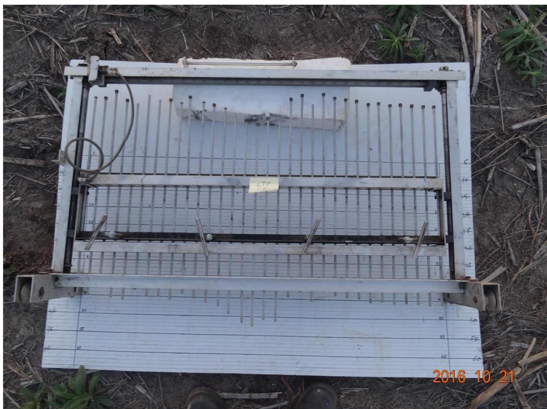
**Figure A3.4: Profile meter used to measure soil surface roughness and rut depth.**
