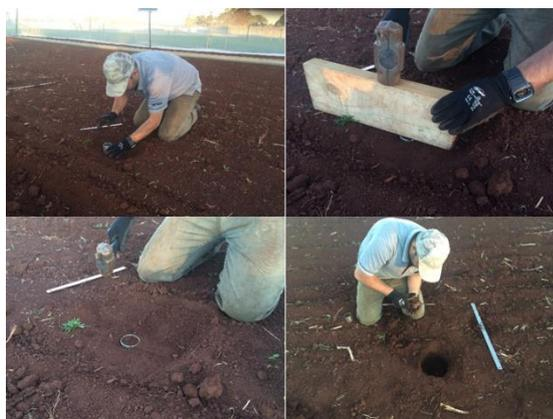
**Figure 3.2: Procedure of bulk density sampling**
