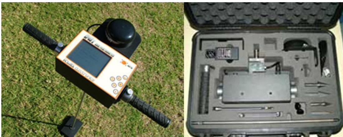
Figure A3.2: Rimik Penetrometer used to measure the penetration resistance of studied soils
