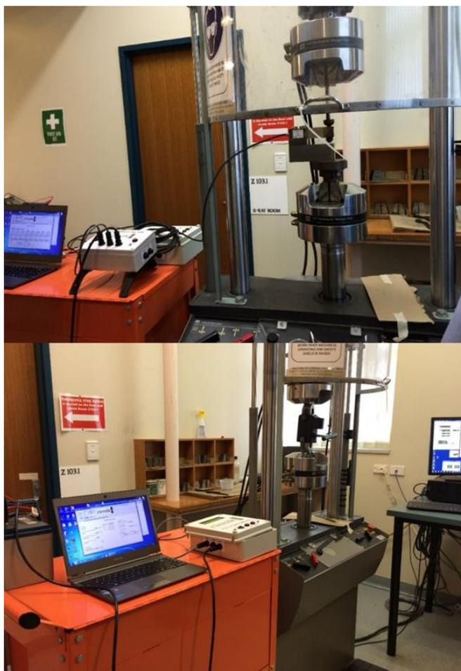
Figure 3.5: Calibration procedure for transducers (top) and pullmeter (bottom)
