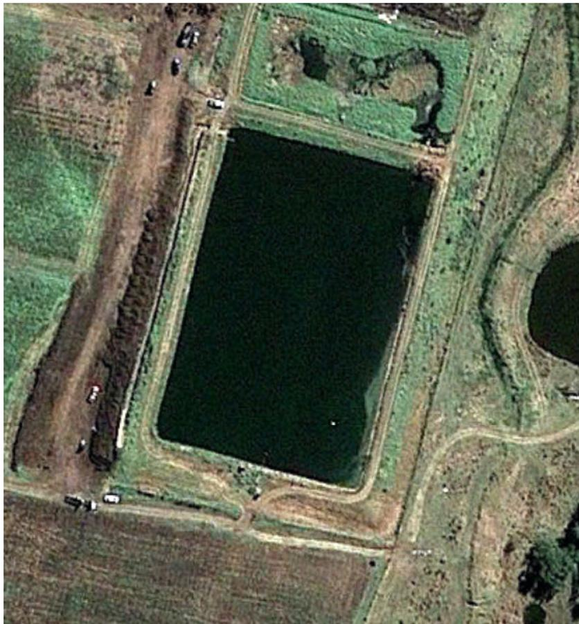
Figure 9.2: ‘Google Earth’ satellite image of the rectangular ring tank storage used in this demonstration. The storage is located at Amberley in Queensland and has a width of 300 meters and a length of 460 meters, which is a surface area of 13.8 ha.
