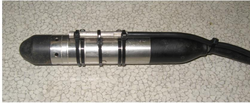
Figure A.2: Druck 4030 pressure sensitive transducer (Craig et al. 2005b)
