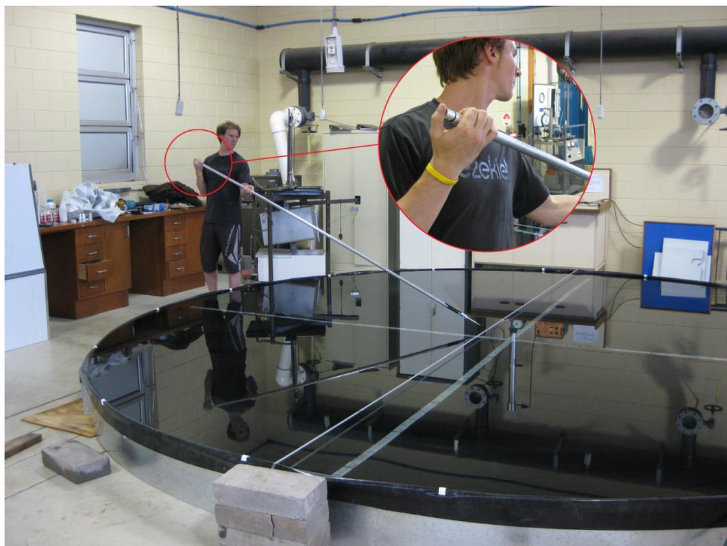
Figure 5.4: 6 m diameter water tank (lined with a black polyethylene liner) used for spreading rate tests. Monolayer is being then applied (by the author) with a calibrated medical syringe fixed to the end of a 3 m long aluminium tube for reach. Another aluminium tube, inside the larger diameter aluminium tube, is used to push down on the syringe plunger to apply monolayer.
