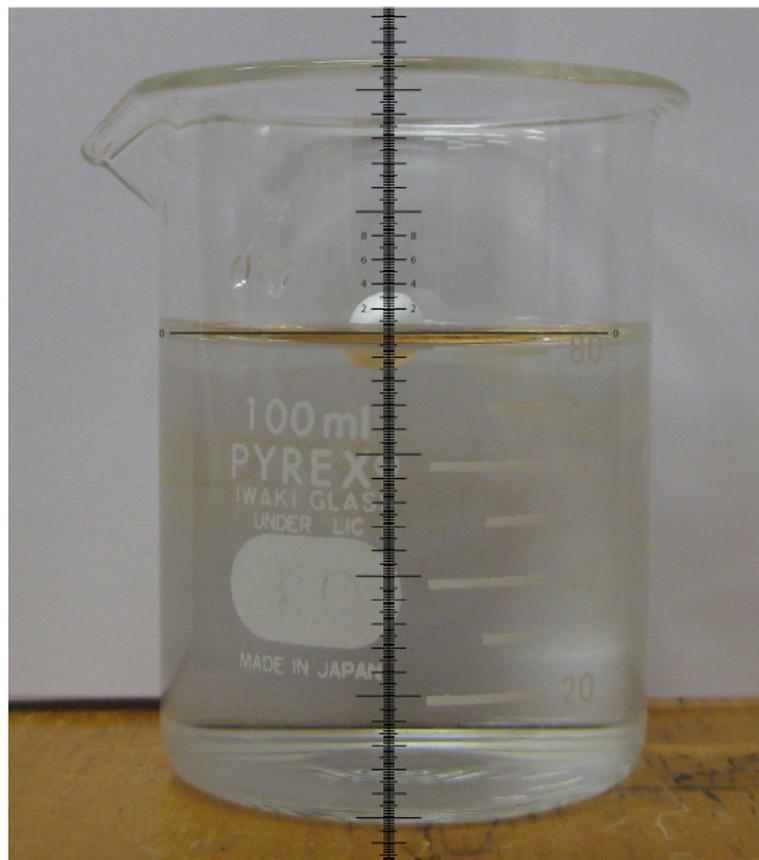
Figure 6.7: The float depth of a 7 mm diameter polyethylene sphere, which were used as an indicator for the drift velocity of the water surface. The centroid of the submerged portion of the sphere was estimated to be 1.75 mm below the water surface.
