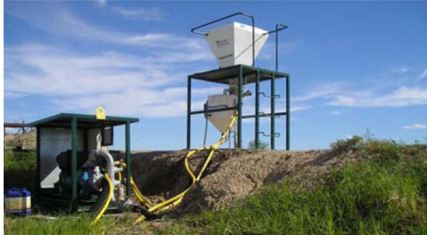
Figure A.17: WaterSavr mixing system designed and built by Bio-Systems Engineering (FSI 2007)
