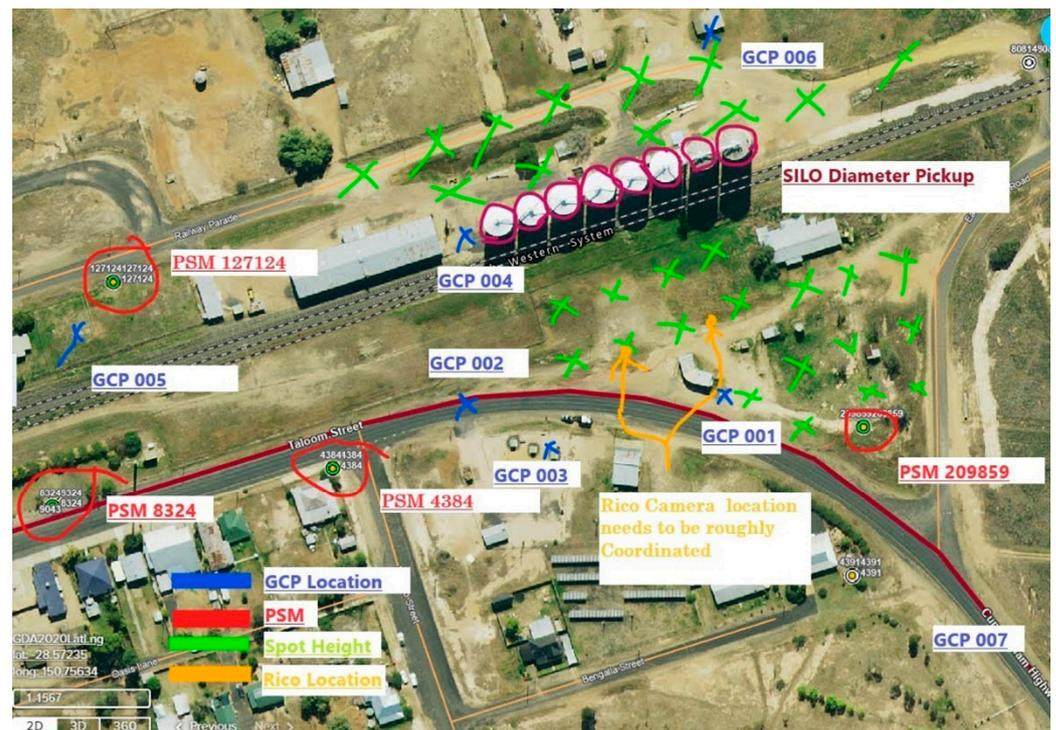
**Figure 4.** Oblique imagery of the Yelarbon Silo, highlighting the project case study location, including GCP, PSM, and Rico Pictures utilised for both photogrammetry and land surveying data collection.
