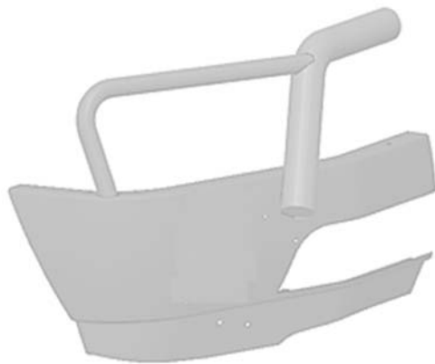
Figure 7.8: Baseline design concept of the bumper replacement type of FPS
