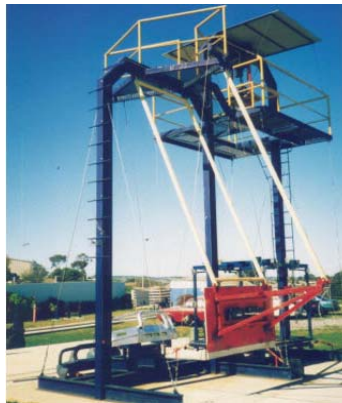
Figure 8.1: Pendulum test rig for the dynamic testing of the bull bar (Adapted from the website of Automotive Safety Engineering)
