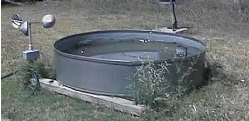
Figure 13 Typical evaporation pan with weeds growing and no bird guard. The pan is also not filled to the top so there will be significant errors associated with the aerodynamics of the lip
