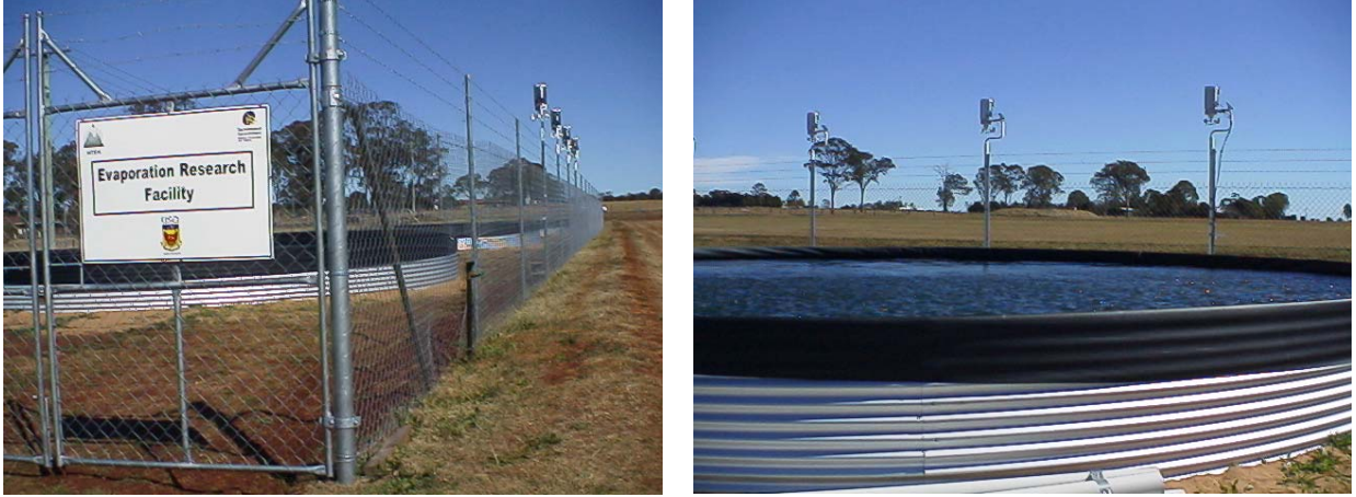
Figure 15 Evaporation Research Facility based at NCEA, USQ. The experimental trial consists of three lined 10m x 0.8m deep tanks which are being used to accurately assess the effectiveness of different evaporation control methods.
