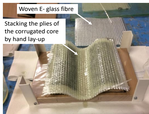
Figure 3.6: The wet-layup technique for manufacturing a single-cell TCS structure made from woven E-glass fibre reinforced composite polymer
