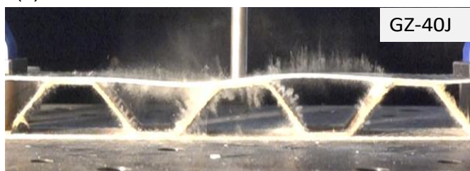
Figure 6.7: TCS structures GG, GK and GZ subjected to 40 J (a) Impact force-time response, and (b-d) Captured image at the end of the impact
