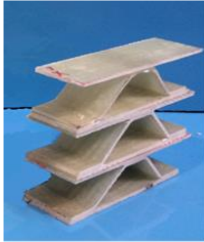
Figure 3.18: The single-cell GC11 TCS structure
