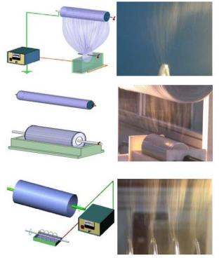
FIGURE. 1 Schematic of disc, cylinder and coil electrospinning systems and electrospinning processes.
