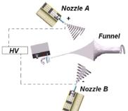
FIGURE 2. Schematic illustration of the basic setup for electrospinning of nanofiber yarns.
