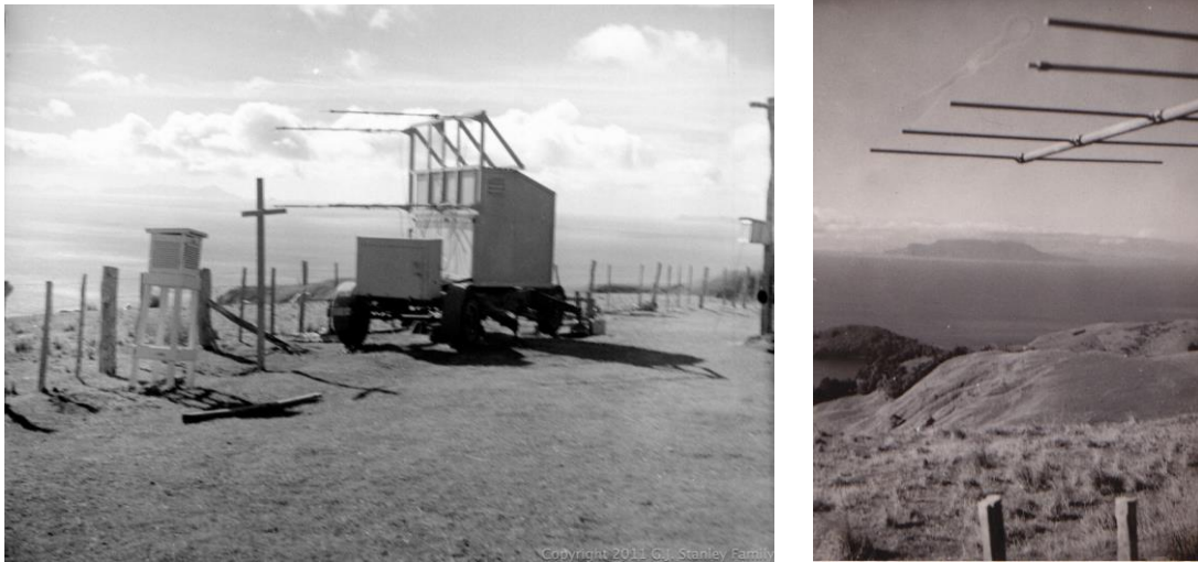
Figure 4.4. The mobile sea interferometer on the Greenwood farm at Pakiri Hill in June 1948. The cabin mounted on the trailer could swivel in azimuth to observe sources rising at different declinations along the horizon. [courtesy: Stanley family]
