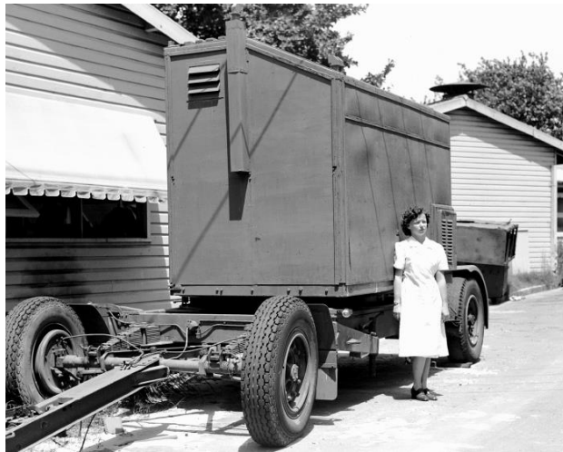
Figure 4.1. The ex-Army radar trailer in the grounds of the Radiophysics Lab. This mobile sea interferometer featured four Yagi aerials, a new 100 MHz receiver, recorders, chronometers, weather recording instruments and all the tools and backup equipment needed to operate reliably at a remote location. [courtesy: RAIA]
