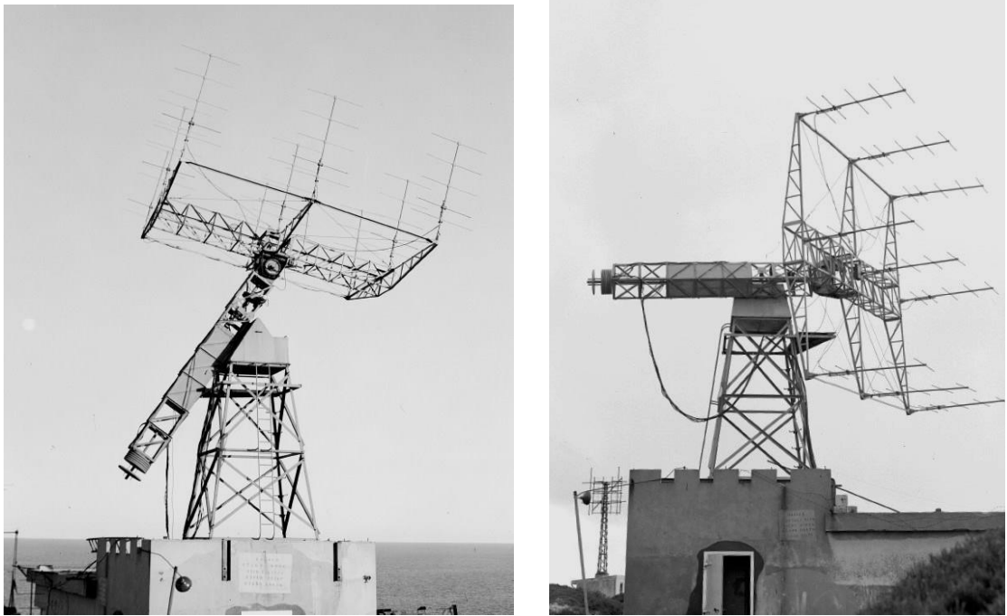
Figure 5.7. The nine-Yagi array was the first of the purpose-built radio telescopes at Dover Heights. (left) The array on its equatorial mounting was used to carry out the first survey of the southern sky at 100 MHz. (right) The array in its sea interferometer mounting. [courtesy: RAIA]
