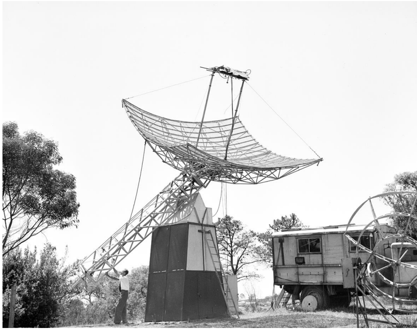
Figure 6.9. The 4.9 \times 5.5 m parabolic antenna at the Radiophysics field station at Potts Hill. In 1950 Jack Piddington and Harry Minnett used the antenna to discover the strong radio source Sagittarius A. [courtesy: RAI]A]
