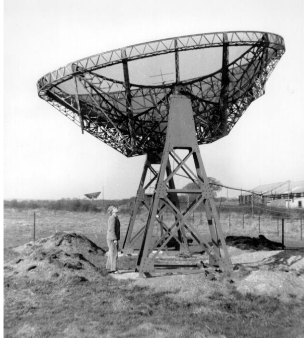
Figure 6.2. Graham Smith with the Cambridge interferometer, consisting of two former wartime Würzburg dishes. Smith used the interferometer in 1951 to measure a precise position for the Cygnus A source as part of his PhD thesis. It was the beginning of a distinguished career for Smith. In 1982 he was appointed Britain's Astronomer Royal. [courtesy: Graham Smith; credit: Bruce Elsmore]
