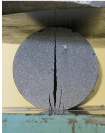
Figure 5.14: Fracture pattern of split tensile sample
