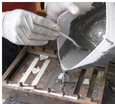
Figure 5.5: Shrinkage testing mould
