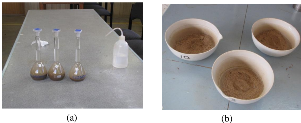
Figure 5.10: Three samples (a) Picnometer + SSD Specimens + Distilled Water, (b) Oven dry samples
