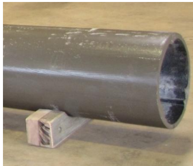
Figure 4.8: Support condition in bending test.
