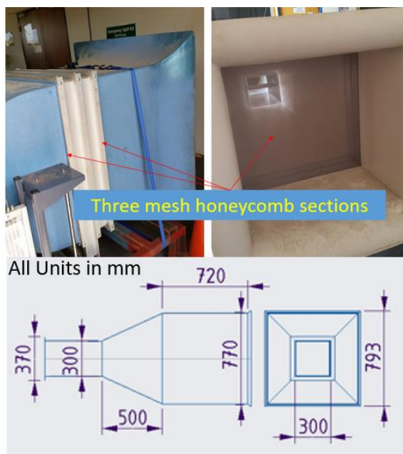
Figure 3-4: Three mesh-wire sections in WT entrance section
