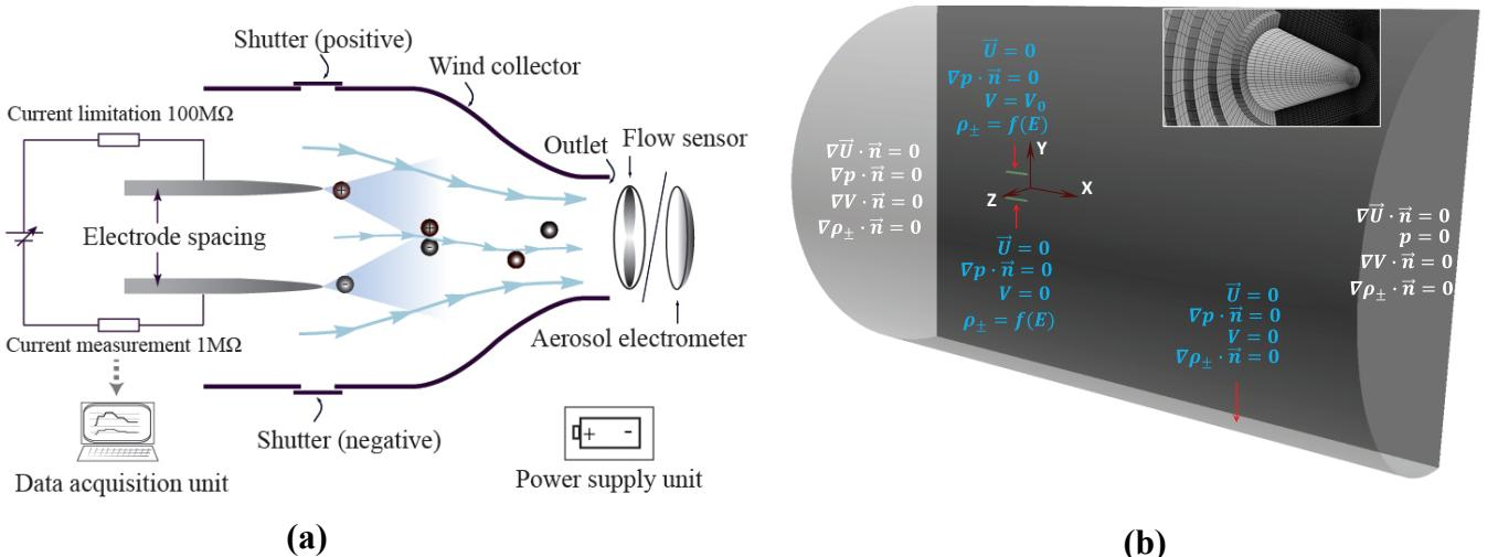
**Fig. 1. Bipolar discharge ion wind generator. (a) Experimental setup. (b) Numerical simulation model, a cylindrical domain with diameter and length of ten and twenty times of electrode separation; the inset shows magnified view of mesh at pin tip.**
