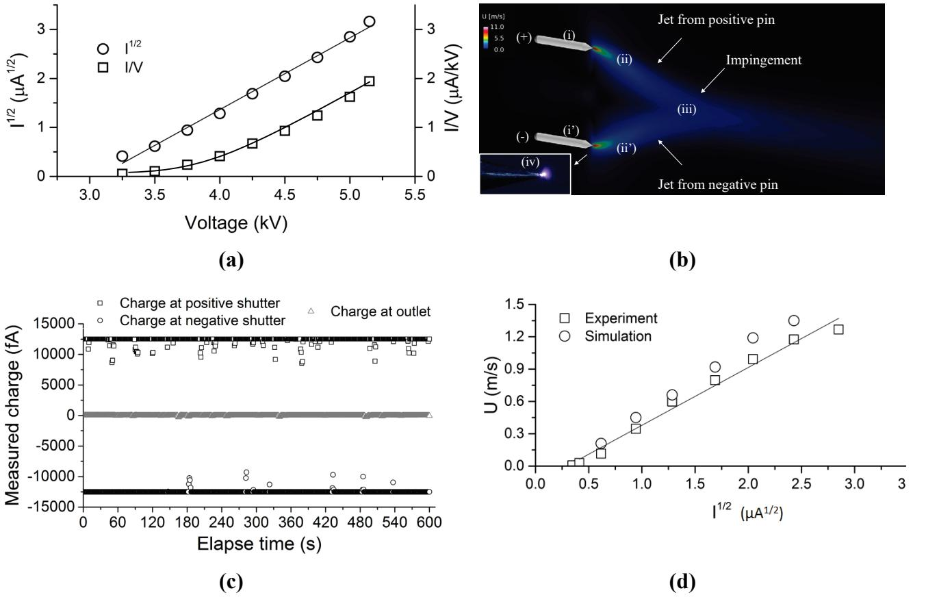
**Fig. 2.** Result for pin tip SR = 15  $\mu\text{m}$ . (a) Voltage – current for electrode separation of 6 mm. (b) Velocity field simulation of the ion wind generation with parameters given in Fig. 2a. (i) & (i') pin tips; (ii) & (ii') jet of ion clouds; (iii) impingement point and (iv) glowing corona image taken at negative pin tip with applied voltage of 4.5 kV and discharge current of 4.0  $\mu\text{A}$ . (c) Charge measurement results. (d) The ion wind velocity plotted versus  $\sqrt{I}$ .
