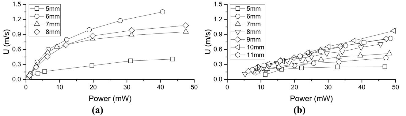
**Fig. 4.** Velocity of ion wind  $U$  plotted with the applied power with (a) pin tip  $\text{SR} = 15 \mu\text{m}$  and a range of electrode separations from 5 to 8 mm; and (b) pin tip  $\text{SR} = 80 \mu\text{m}$  and a range of electrode separations from 5 to 11 mm.
