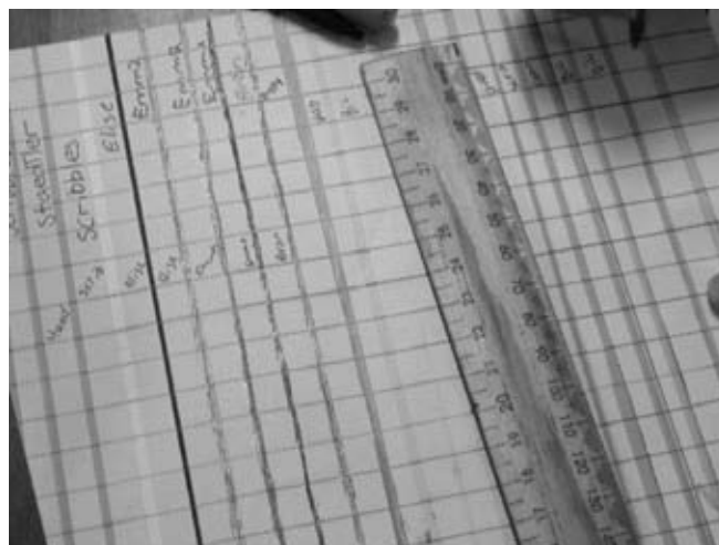
Figure 1) Manufacturing and testing for suitable ink that could be used as a UV dosimeter with a primary school aged group. Students tested many different types of highlighters and pens in ruling up this A4 sheet.
